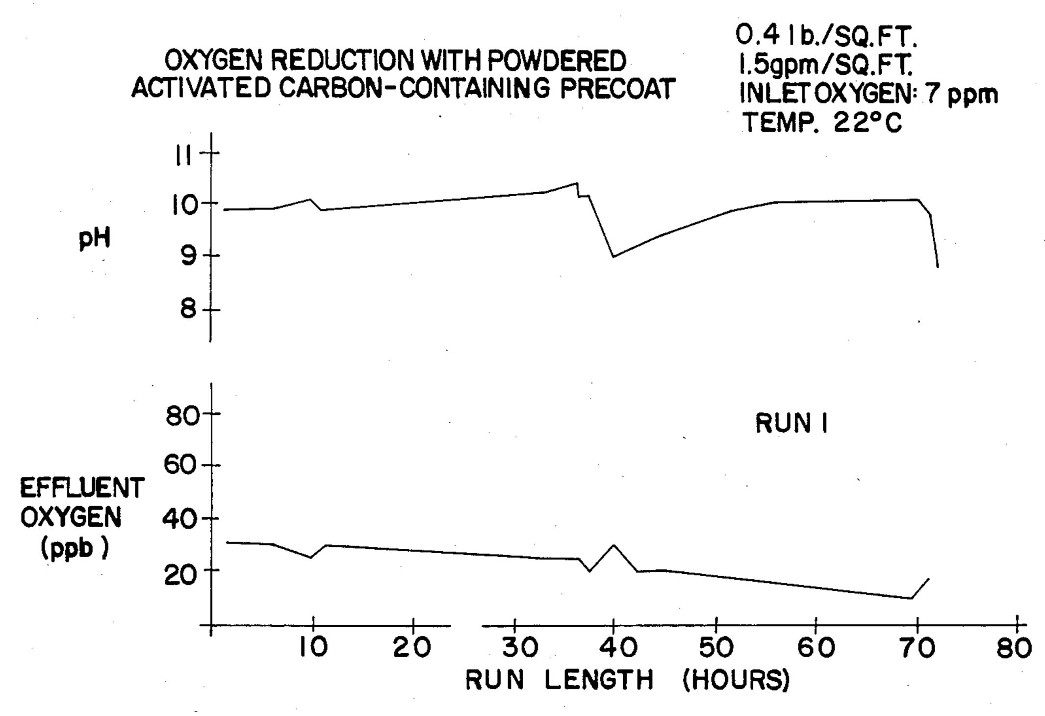
OXYGEN REDUCTION WITH POWDERED ACTIVATED CARBON-CONTAINING PRECOAT 0.41b./SQ.FT. .5gpm/SQ.FT. INLET OXYGEN: 7ppm TEMP. 22°C
