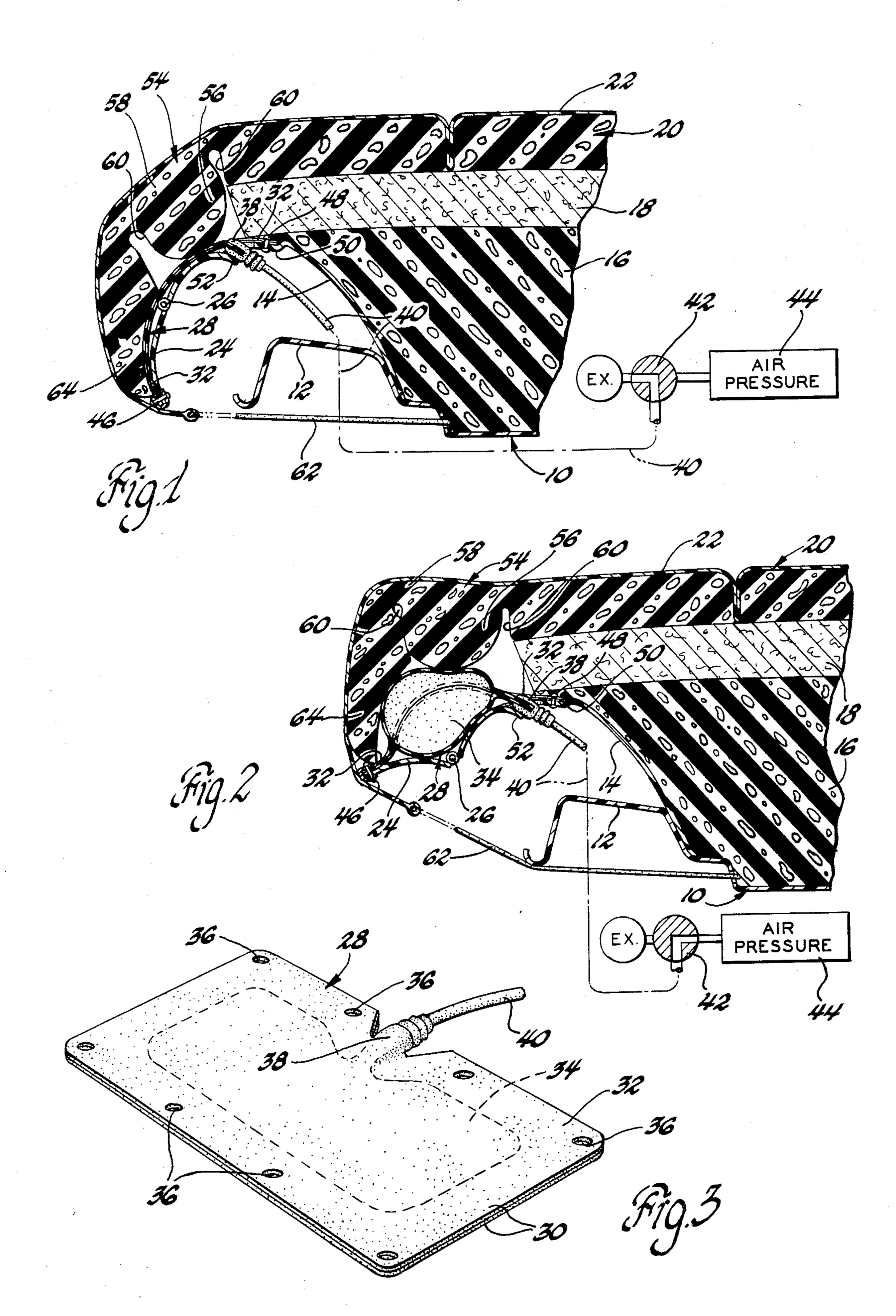
FIG. 1 is a sectional view of the forward edge portion of a vehicle seat cushion embodying an inflatable thigh support according to this invention, with the thigh support being shown in a deflated condition.
