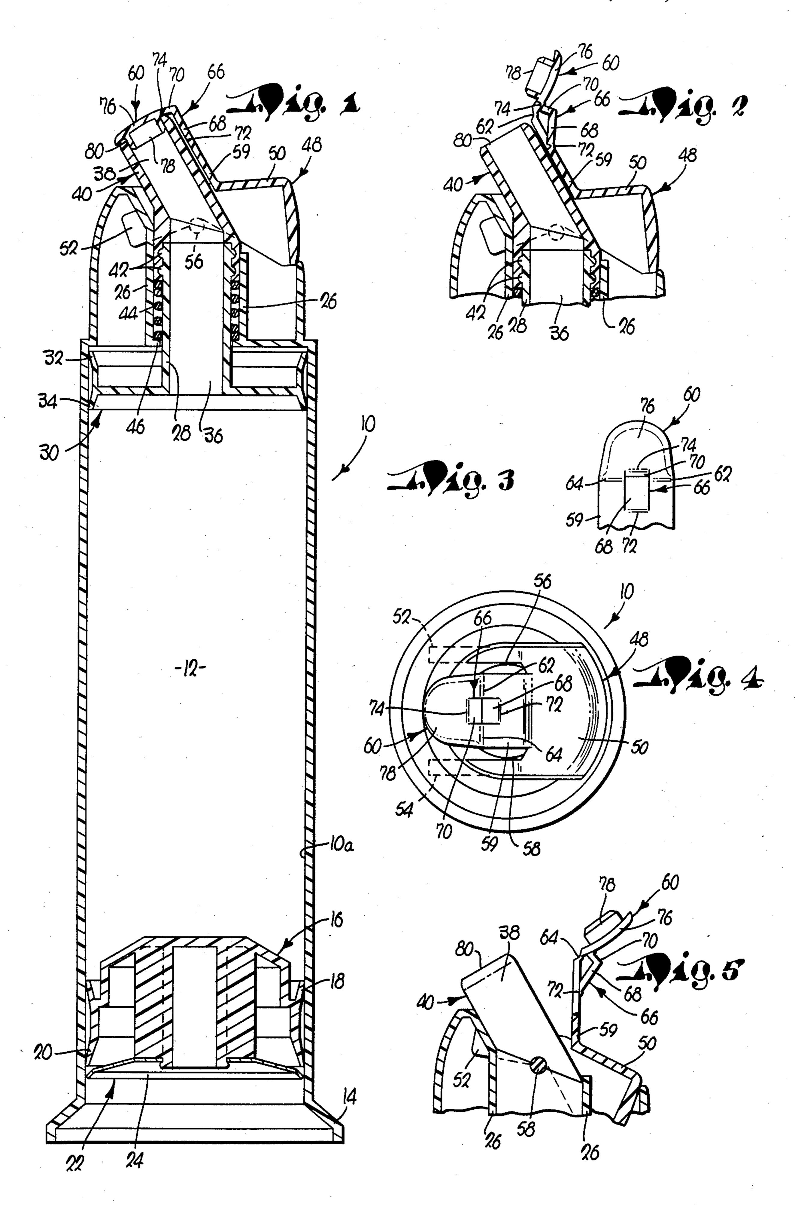
SNAP-ACTION ORIFICE SEALING PLUG FOR
