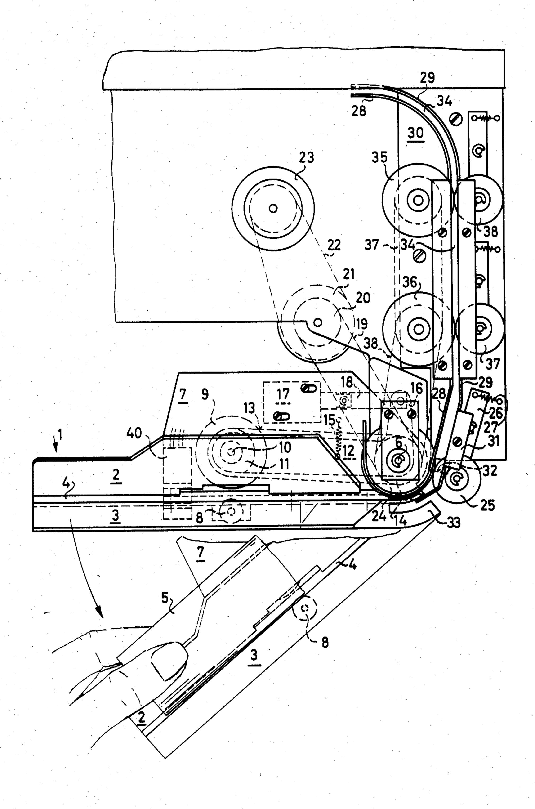
ported a further document transport means on the same pivoting axle as the feed chute so that these further transport means can then assume the transport function
