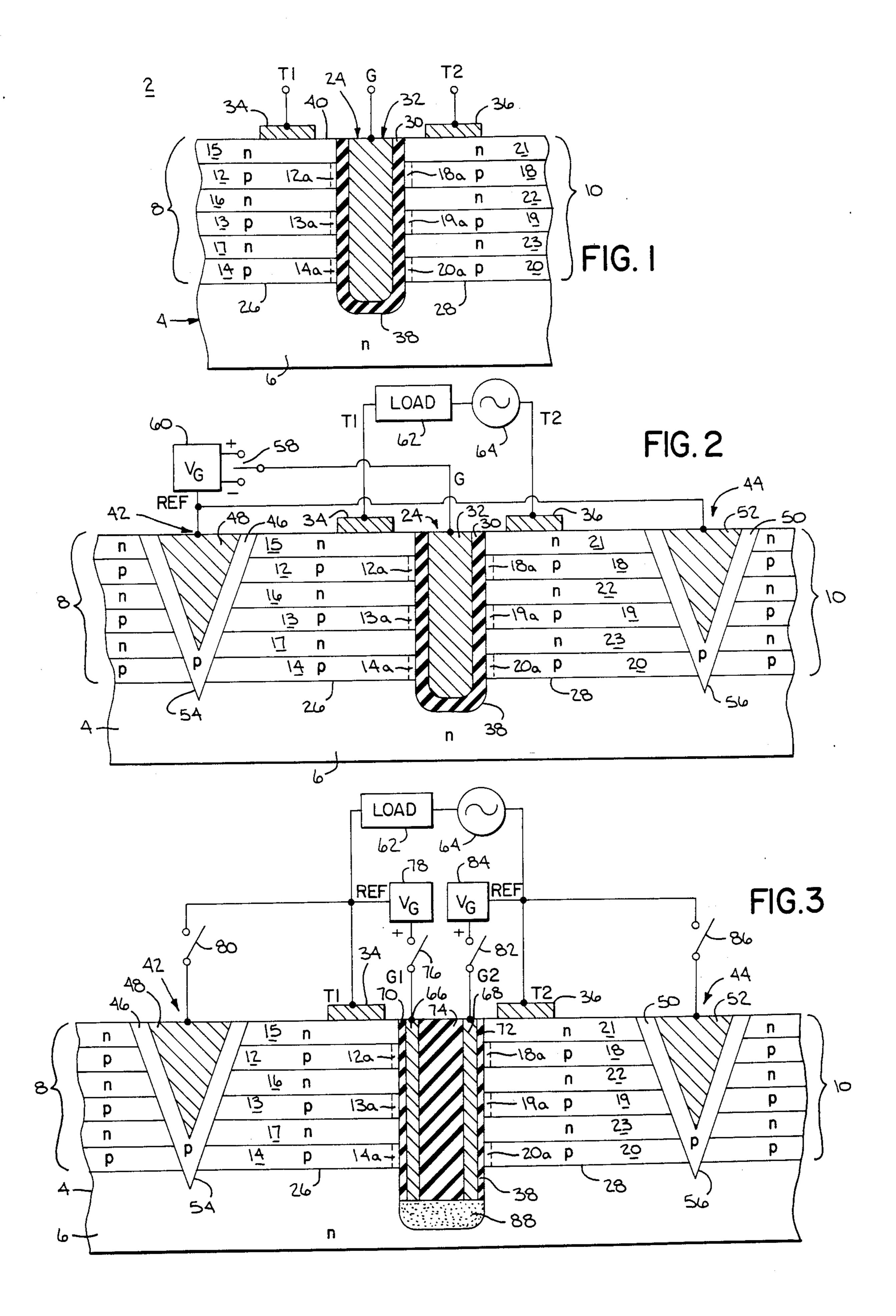
ductor material, such as n type, and forms a first junction 26 with channel-containing region 14 of first stack 8, and forms a second junction 28 with channel-containing region 20 of second stack 10...
