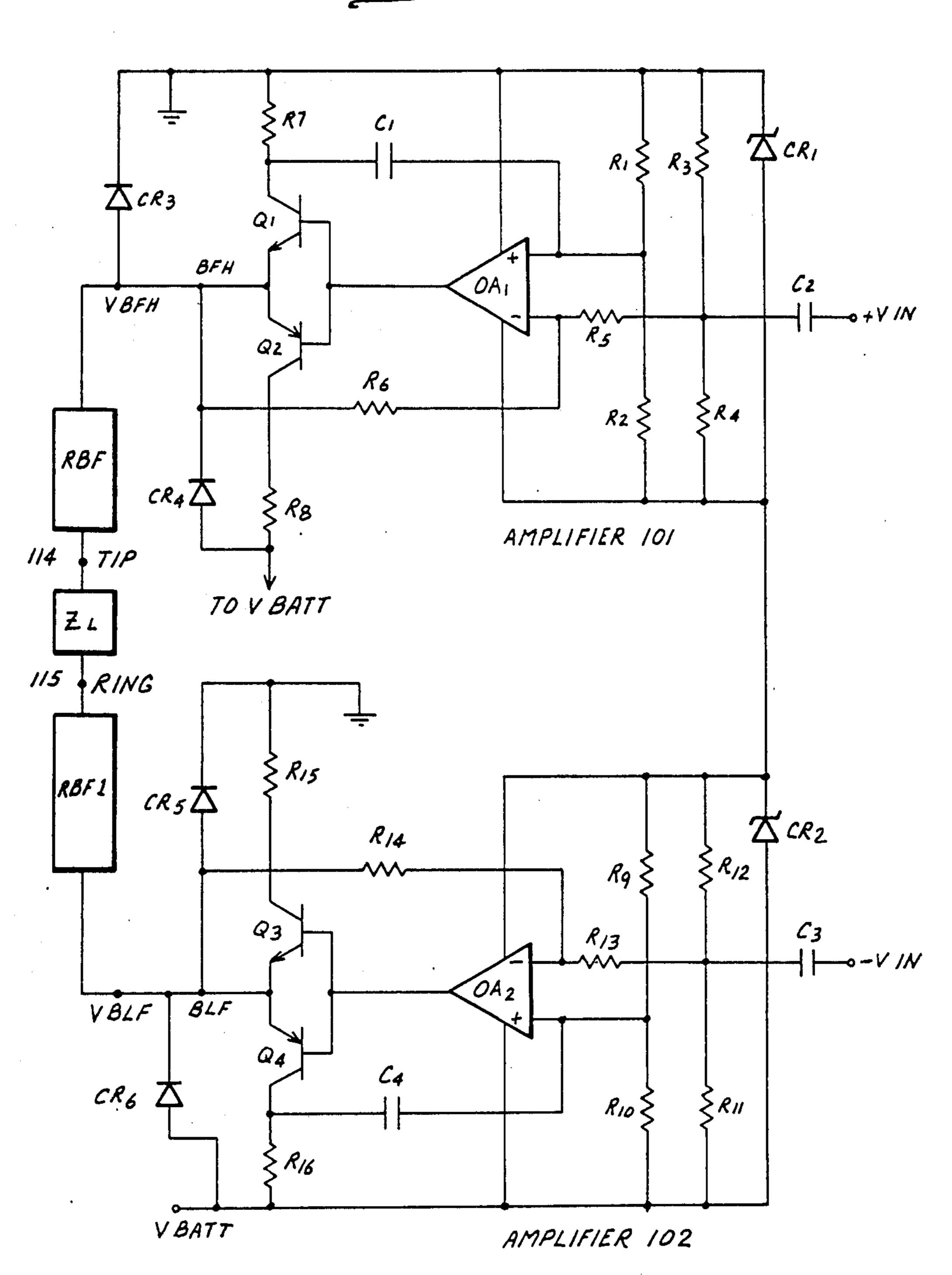
comprises a set of serially connected diodes having a central node connected between a feed resistor and the output terminal of the power amplifier.
