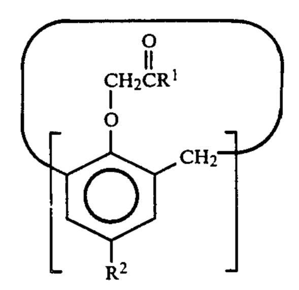
where  $R^1$  is alkyl, alkoxy, substituted alkyl or substituted alkoxy;  $R^2$  is H or alkyl; and n=4, 6, or 8. The compounds may be effectively employed at levels of between about 0.1% and 1% by weight of a cyanoacrylate adhesive composition.
