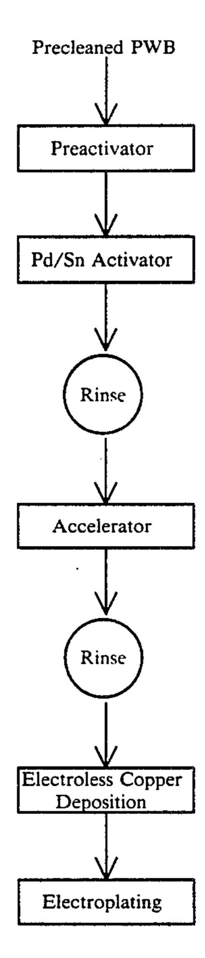
These processed boards may also be photoimaged before the electroplating process. Typically, the deposited copper layer on each through hole wall is about  $1\pm0.2^{60}$  mil thick.
