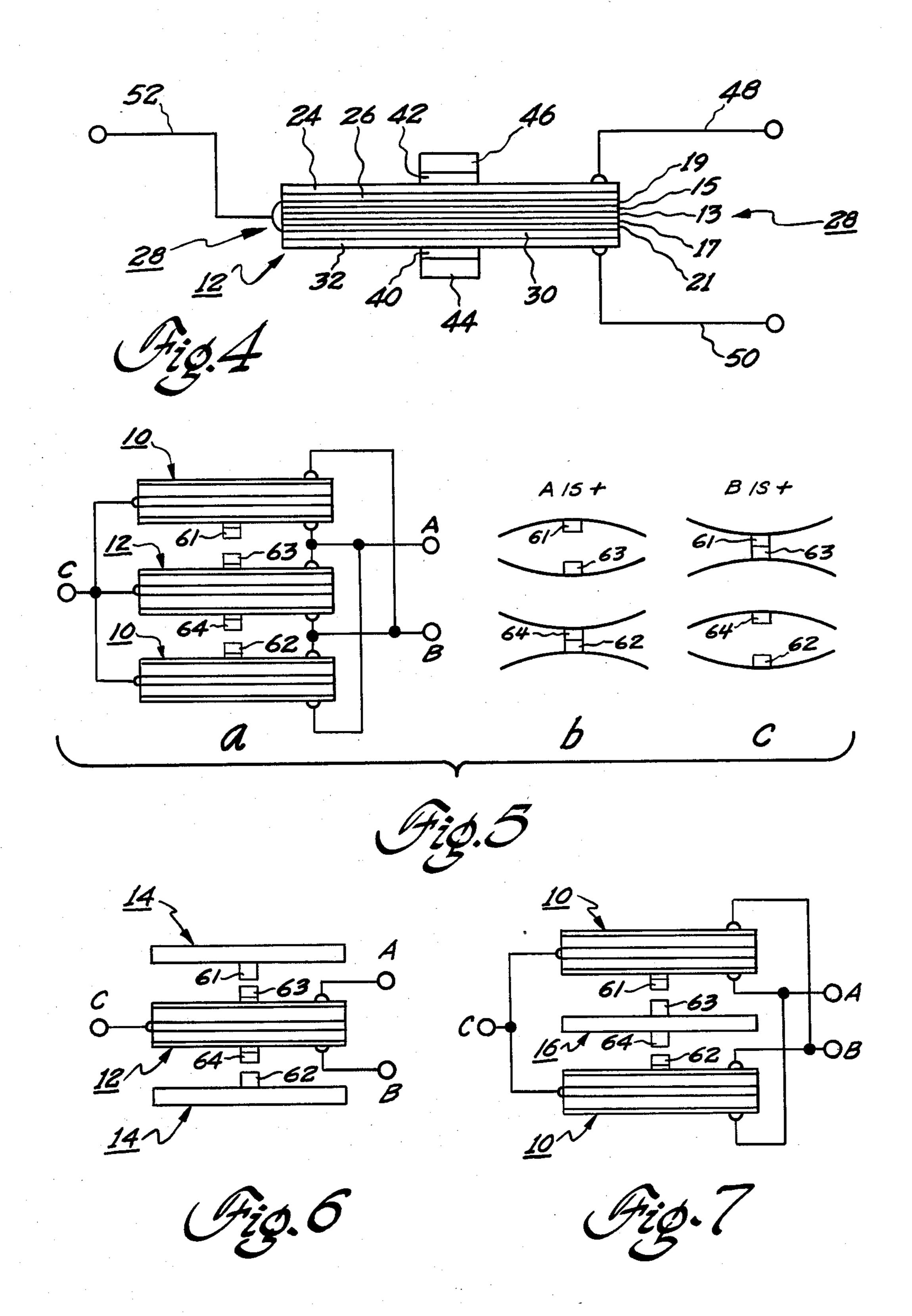
SYNCHRONOUSLY OPERABLE ELECTRICAL CURRENT SWITCHING APPARATUS HAVING INCREASED CONTACT SEPARATION IN THE OPEN POSITION AND INCREASED CONTACT CLOSING FORCE IN THE CLOSED POSITION
