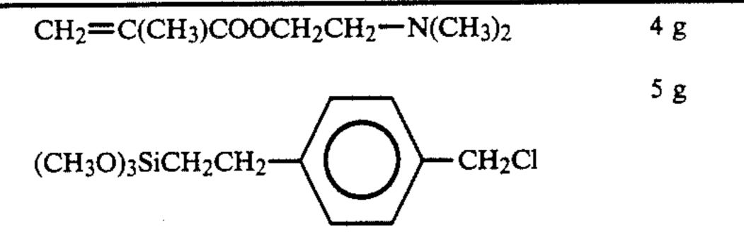
unsaturated amine. The silica was again thrown into a Henschel mixer, and dimethyldichlorosilane was sprayed onto said silica under stirring to a quantity of 2%. Then, the same treatments as in Example 1C were applied. The hydrophobicity was found to be 50.
