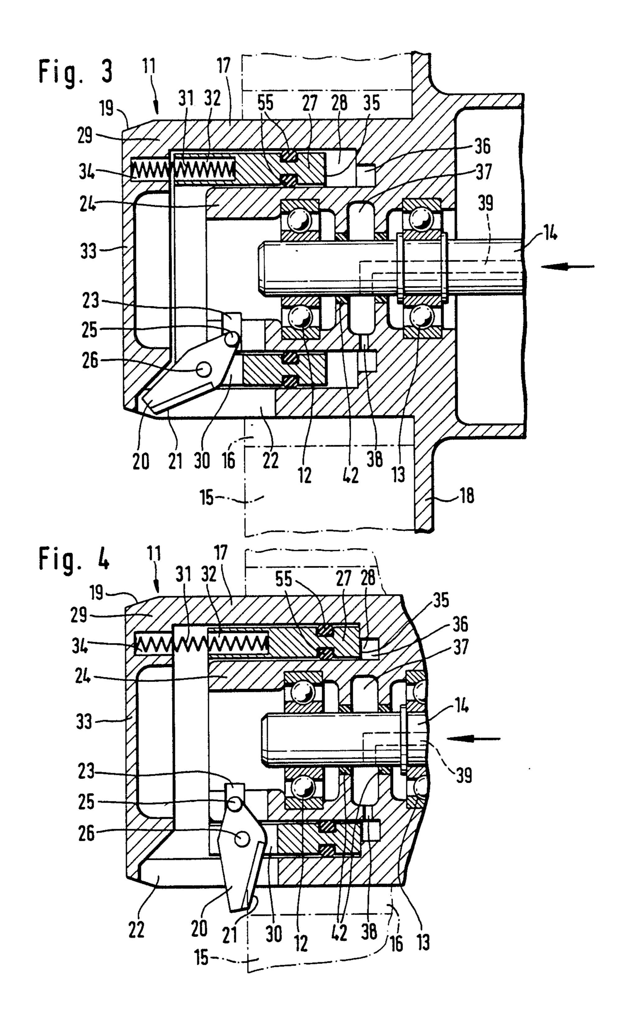
Further features of the invention relate to the design of the clamping claws and to the actuation of these and to the mounting of the hub.
