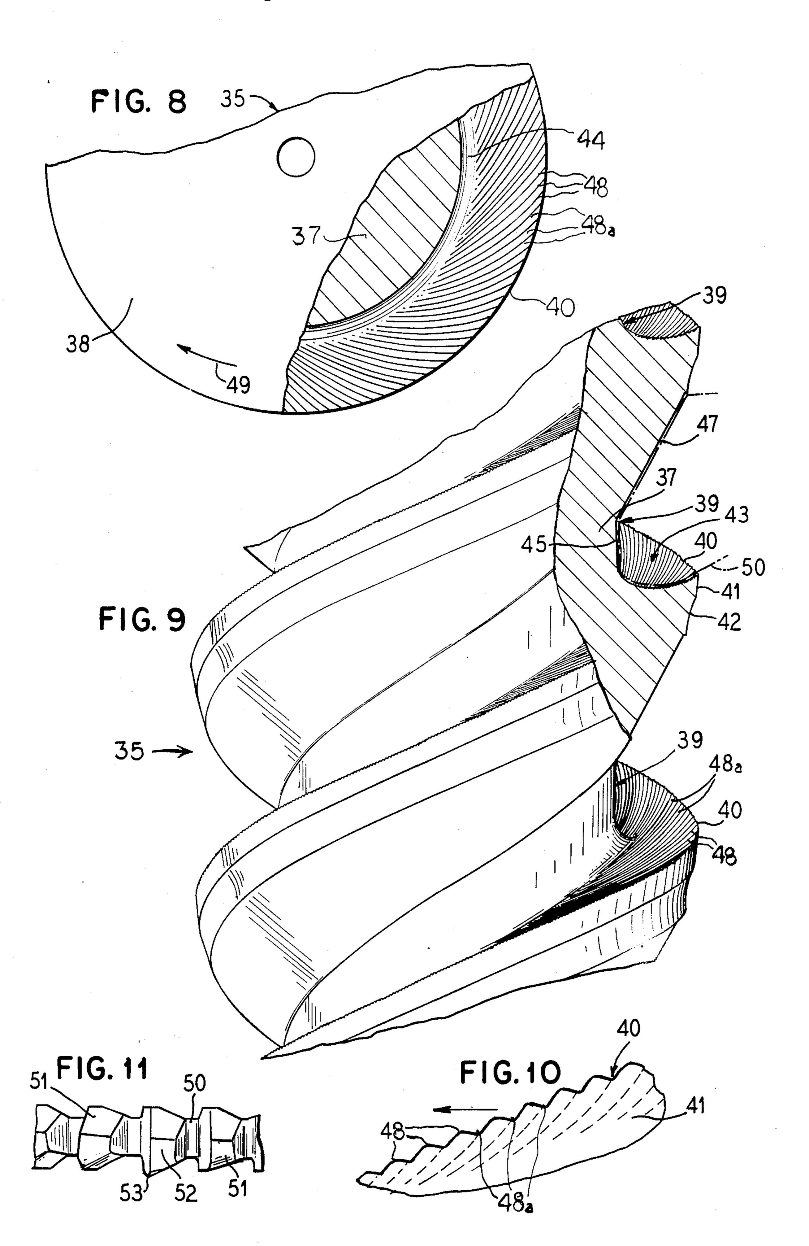
the workpiece, and in combination with said surfaces, forming tightly curled substantially straight elongated chips substantially as long as the depth of cut in the workpiece.
