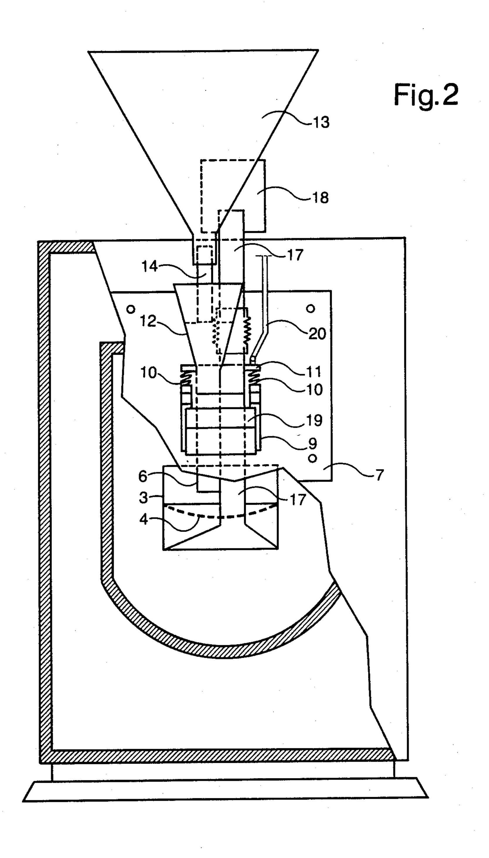
VIBRATING GRATE IN A HEATING BOILER
