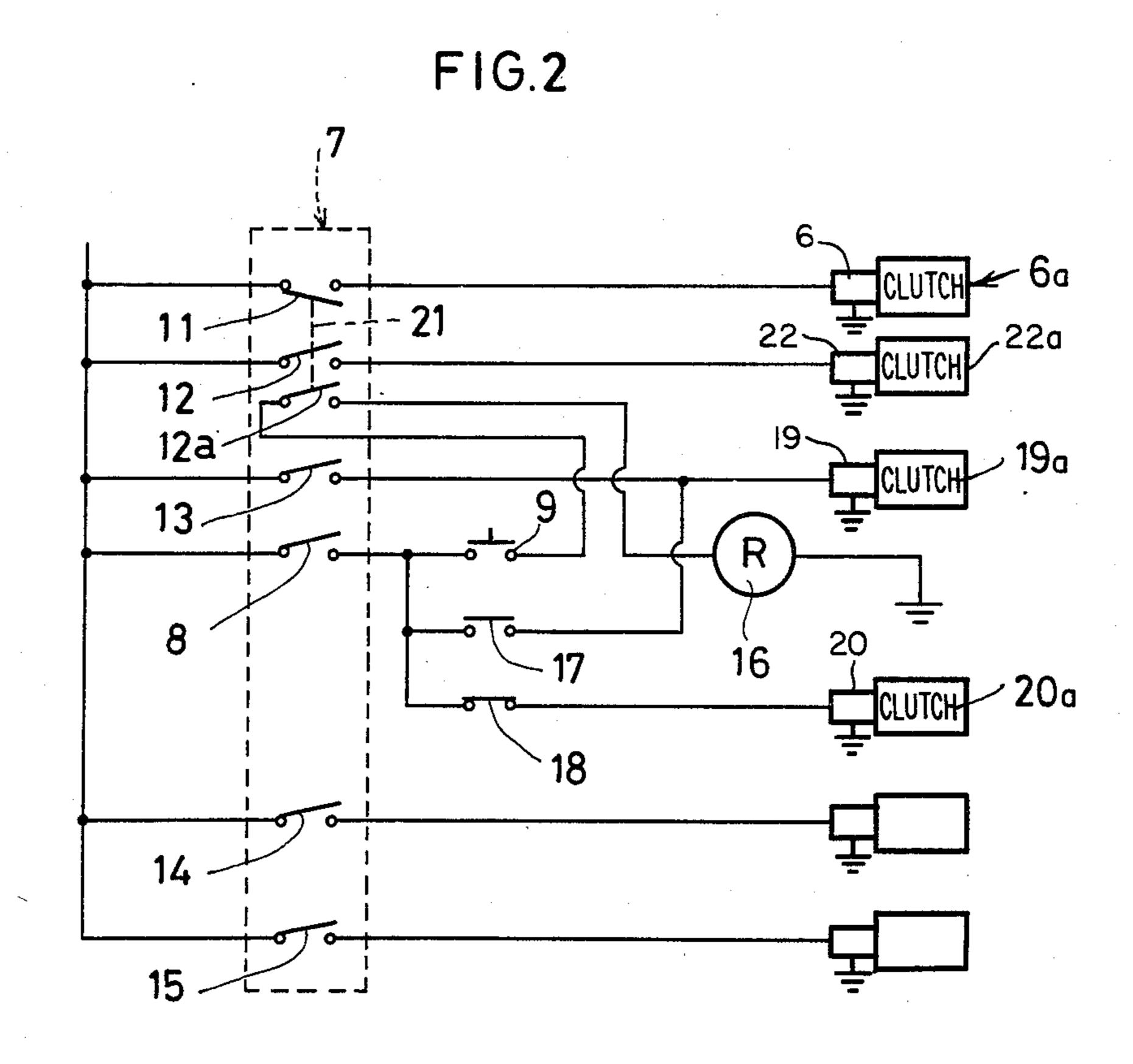
17 and a B contact 18, a first speed solenoid valve 19, and a second speed solenoid valve 20 are also provided.
