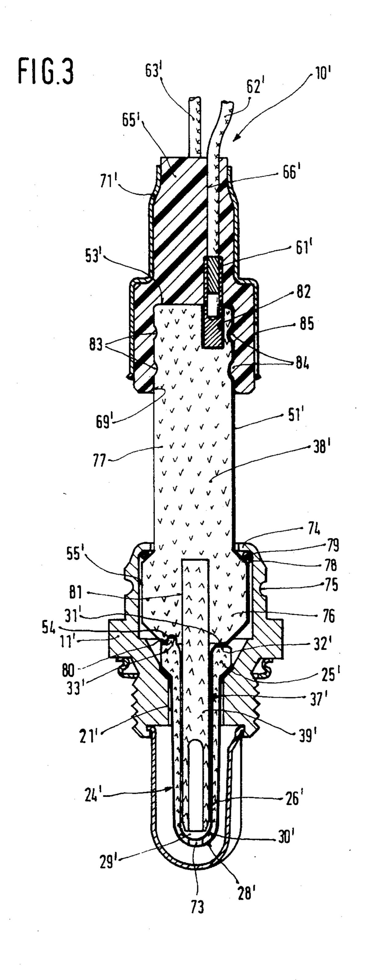
FIG. 3 is a longitudianl section through a second embodiment of an oxygen measuring sensor, again on a magnified scale.
