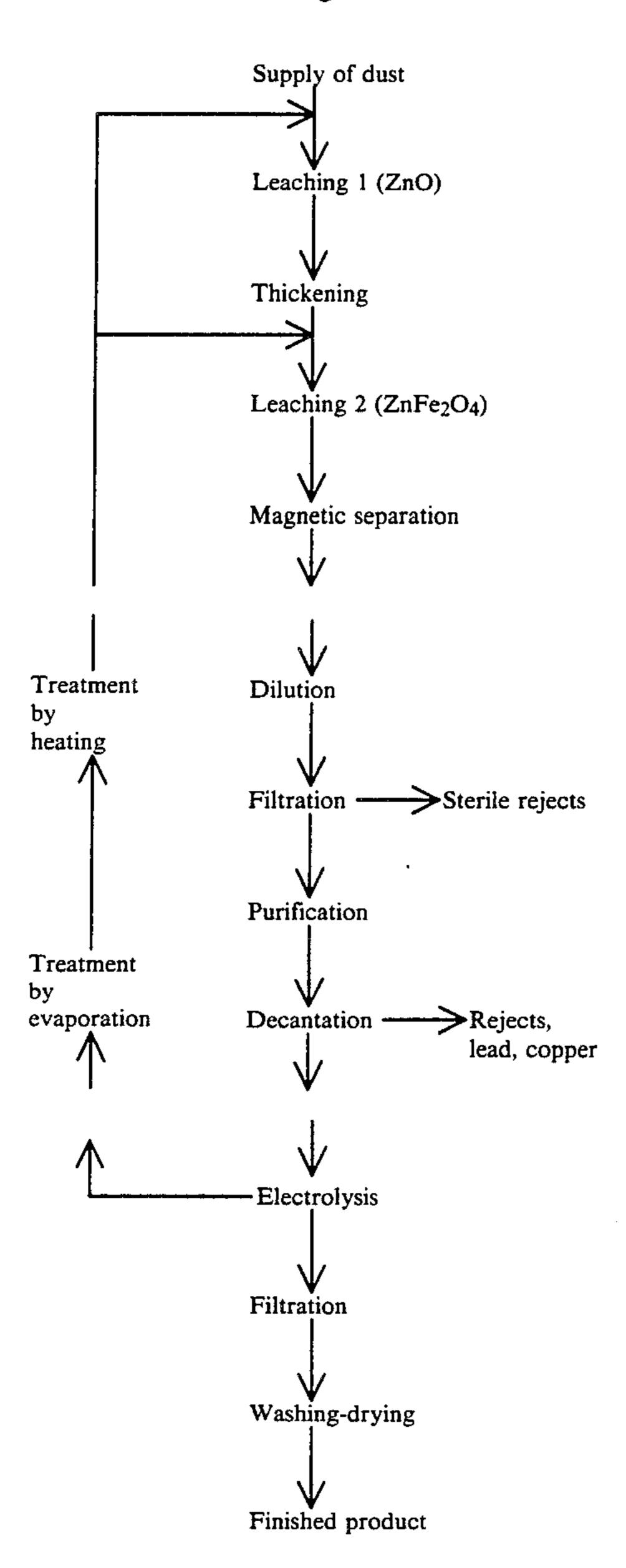
Experience has shown that almost all the zinc oxide is placed in solution by the first leaching. Furthermore, the very ferromagnetic character of the zinc ferrite makes it possible, by a low intensity magnetic separation, to isolate it and recycle it for the second leaching. In this way, 97.5% of the zinc contained in the dust is placed in solution and the sterile rejects contain less than 1% zinc (0.85%).
