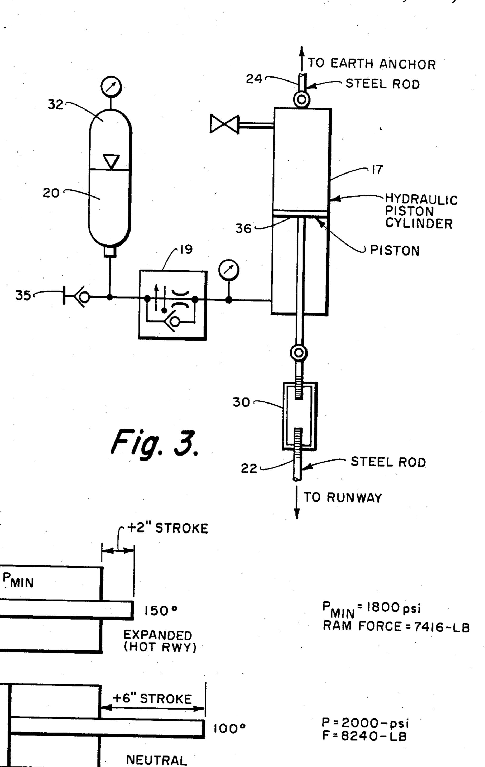
CYLINDER CAPACITY = ± 6 INCH STROKE LOAD MAINTAINED BY TENSION UNIT VS.-RUNWAY EXPANSION/CONTRACTION
