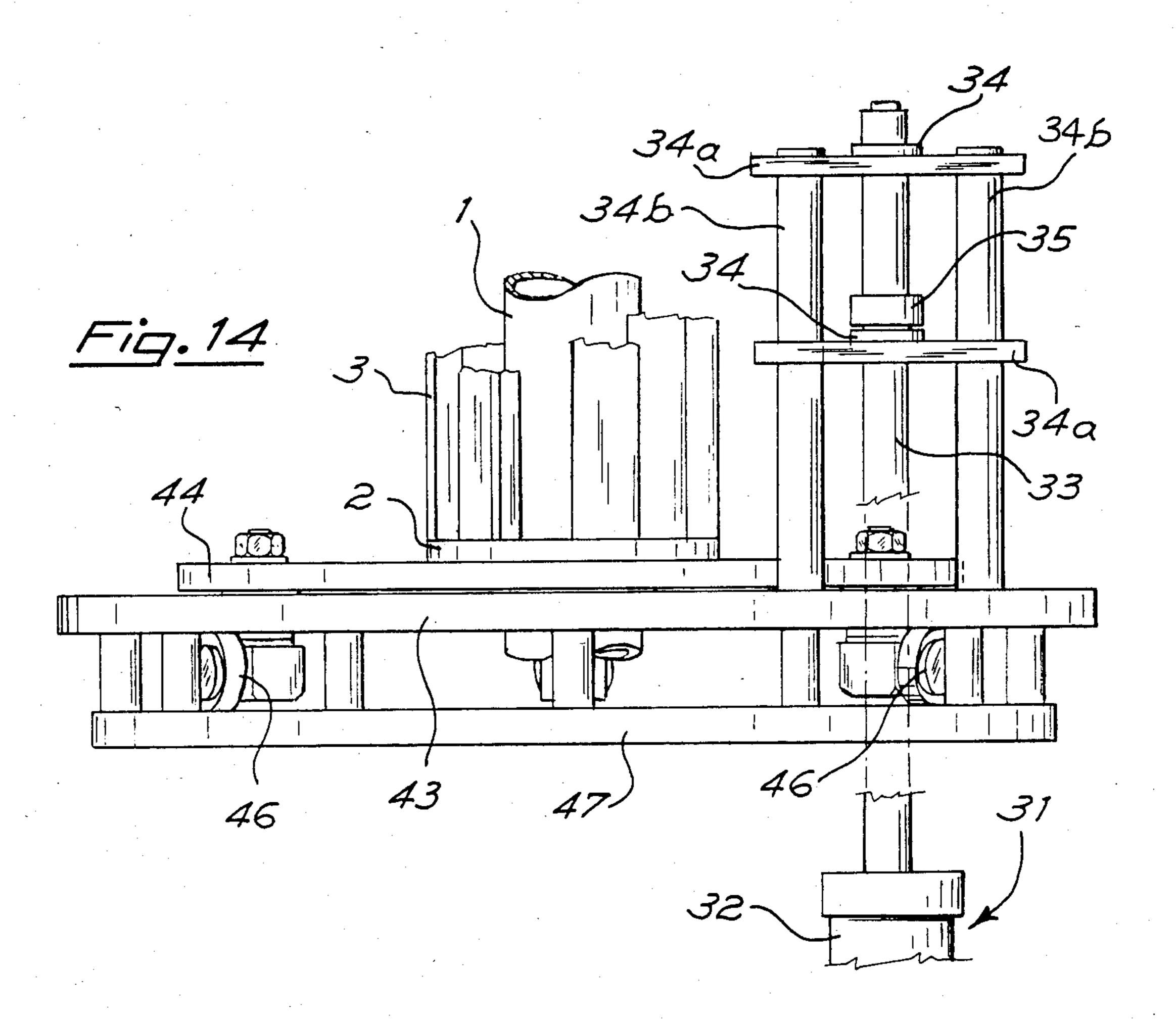
CONTROL DEVICE FOR THE OPENING AND CLOSING OF THE METAL BAR SLIDING GUIDES IN AN EQUIPMENT FOR THE FEEDING OF METAL BARS TO A MULTIPLE-SPINDLE LATHE 5
