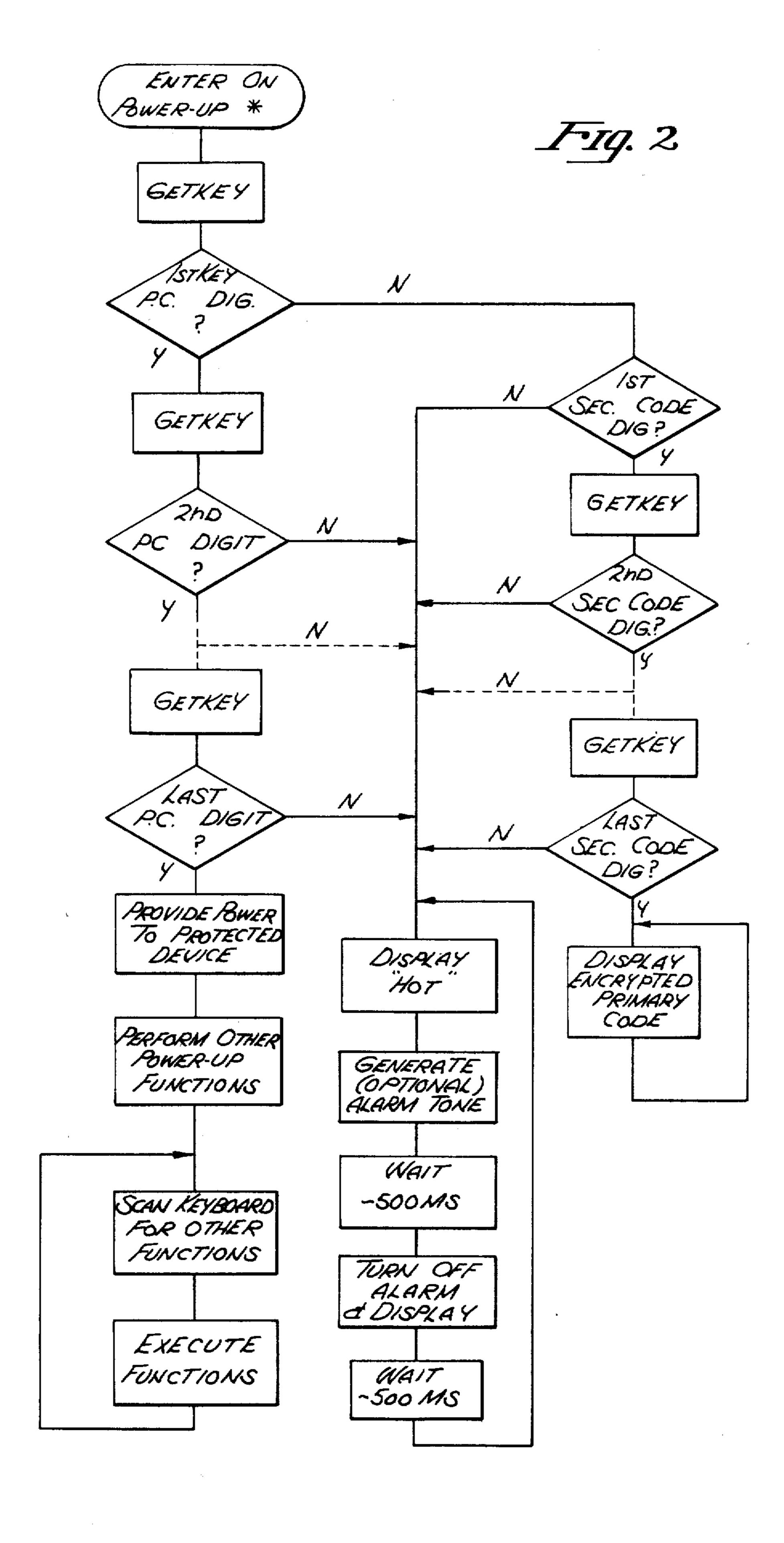
ELECTRONIC SECURITY SYSTEM FOR EXTERNALLY POWERED DEVICES
