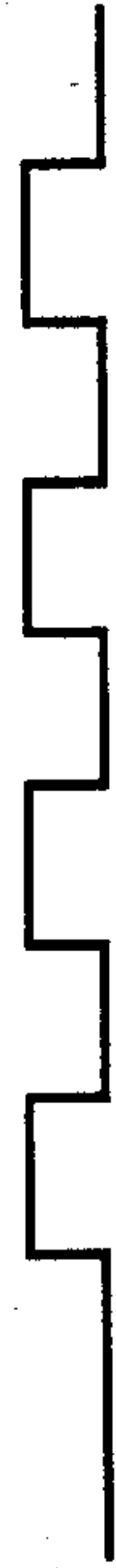
VOLTAGE ON SEGMENTS S2, S4~S27, S29, S32
