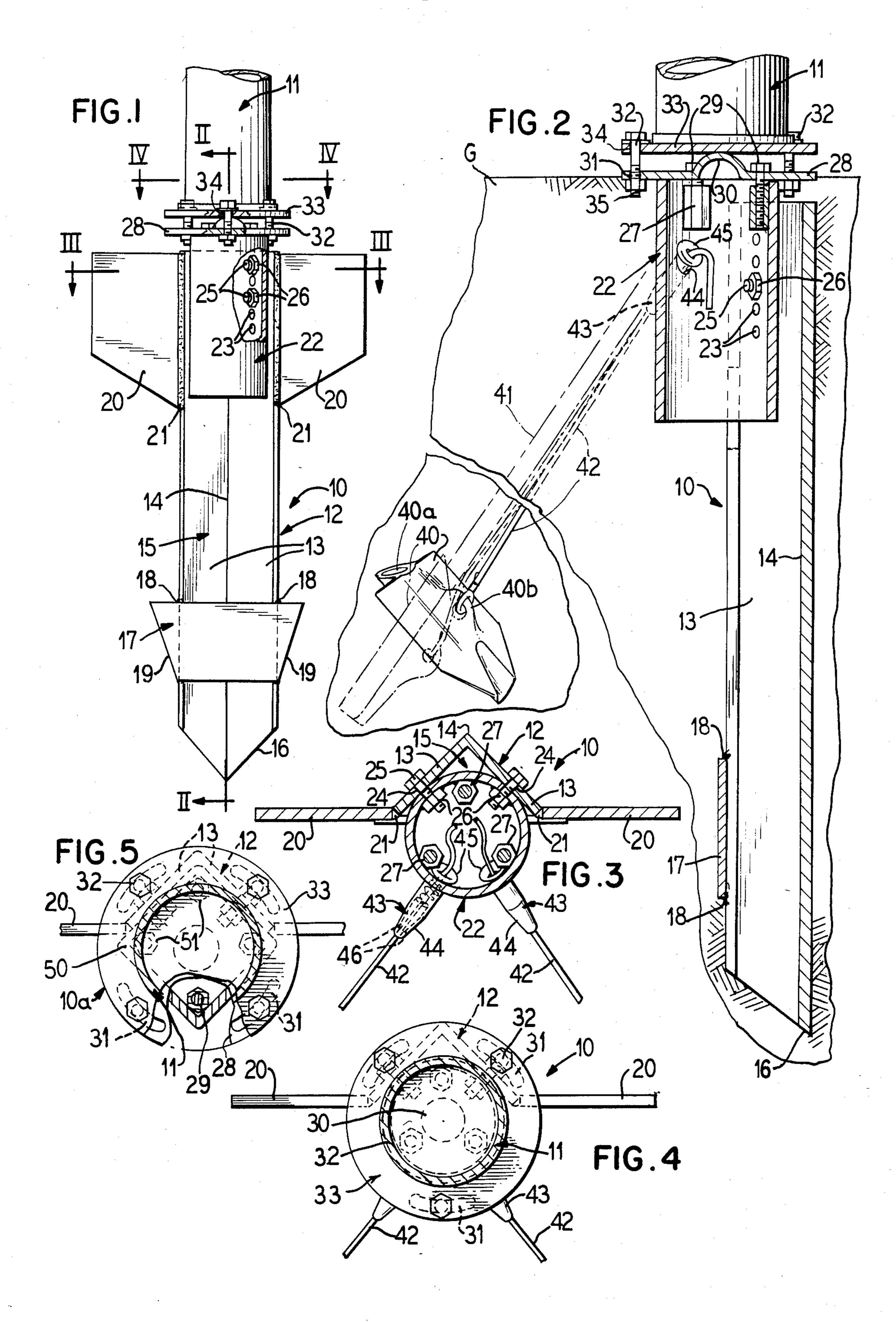
Ground anchored cable guy lines may be attached to the tube to further secure and retain the angle iron leg in the ground.
