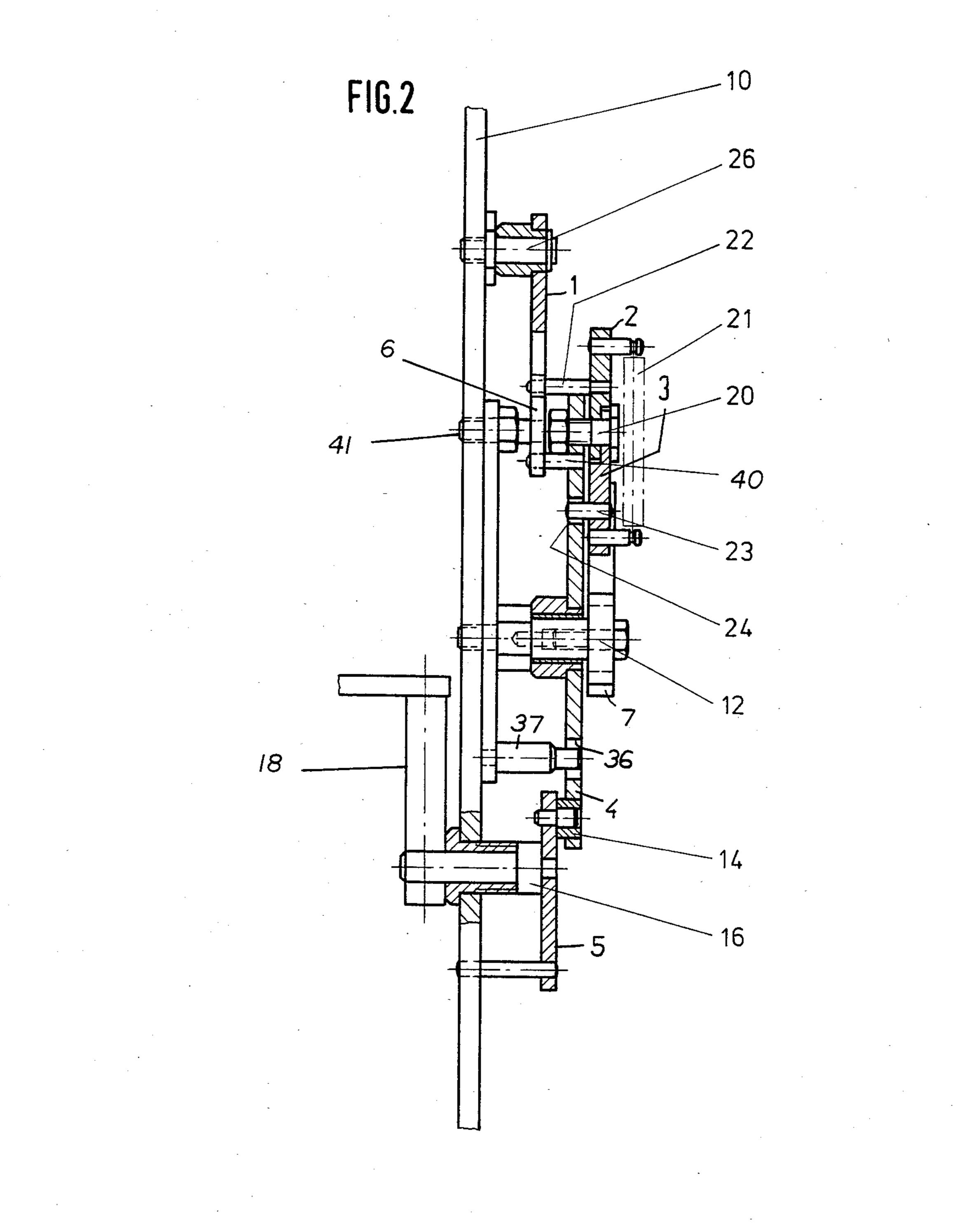
MECHANISM FOR SELECTIVELY CONVERTING A CONTINUOUS ROTARY MOVEMENT TO A PHASE-RELATED SINGLE PIVOTING MOVEMENT OF A CONTROL LEVER
