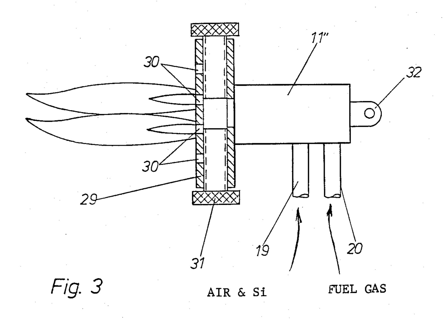
APPARATUS AND METHOD FOR APPLYING A SILICON OXIDE-CONTAINING ADHESION-PROMOTING LAYER ON METALLIC DENTAL PROSTHESES
