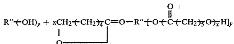
where  $R''$  denotes the residue of a polyhydric alcohol after subtracting  $y$  number of  $-\text{OH}$  groups,  $y$  preferably being 2 or 3 and  $x$  has an average value of from 3 to about 20 and preferably no less than 5. Though higher values of  $x$  are suitable, the high melting points and low solubility of such compounds may require the use of aggressive solvents for dissolution which would damage the plastic substrate to which the coating is applied.
