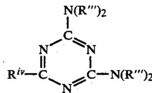
wherein  $\text{R}'''$  is independently selected from H,  $-\text{CH}_2\text{OH}$ , and  $-\text{CH}_2\text{O}(\text{CH}_2)_z\text{H}$ , wherein  $z$  is an integer from 1 to 6, and  $\text{R}''$  is selected from H,  $-\text{OH}$ ,  $-\text{CH}_3$  and  $-\text{N}(\text{R}''')_2$ . Preferably,  $\text{R}''$  is  $-\text{N}(\text{R}''')_2$  and all  $\text{R}'''$  are an alkoxymethyl, particularly, methoxymethyl.
