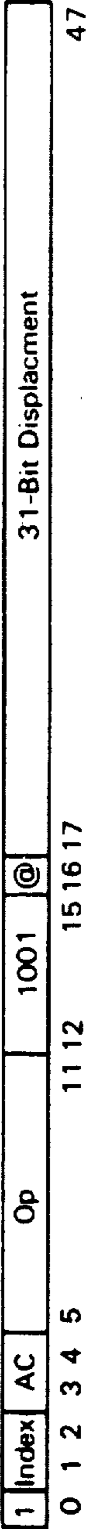
A typical instruction format with a 31-bit displacement (word addressing)
