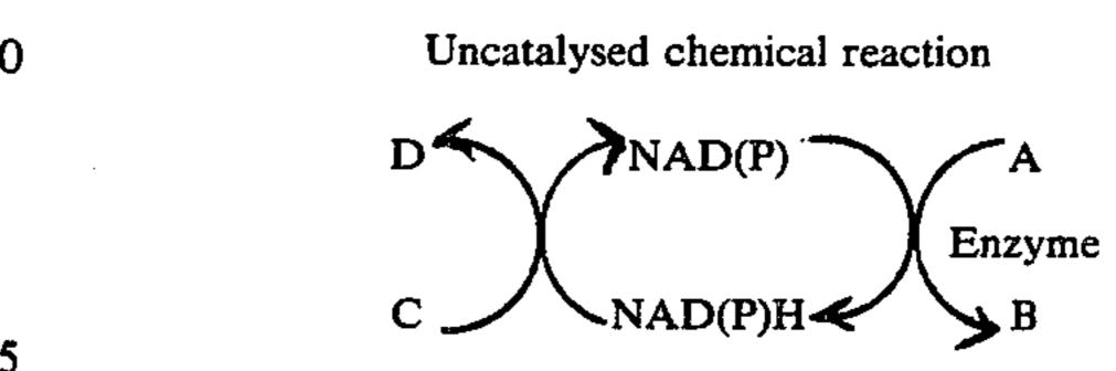
Substances capable of reduction with concommitant oxidation of NAD(P)H are well known, for example, 3'-(4,5-dimethylthiazolyl-2)-2,5-diphenyltetrazolium (MTT tetrazolium) is particularly useful, because on reduction it gives a blue coloured product and, moreover, the results are linear with regard to the NAD(P). A secondary enzyme cycle involving an NAD(P)-/NAD(P)H interconversion may therefore be determined directly.
