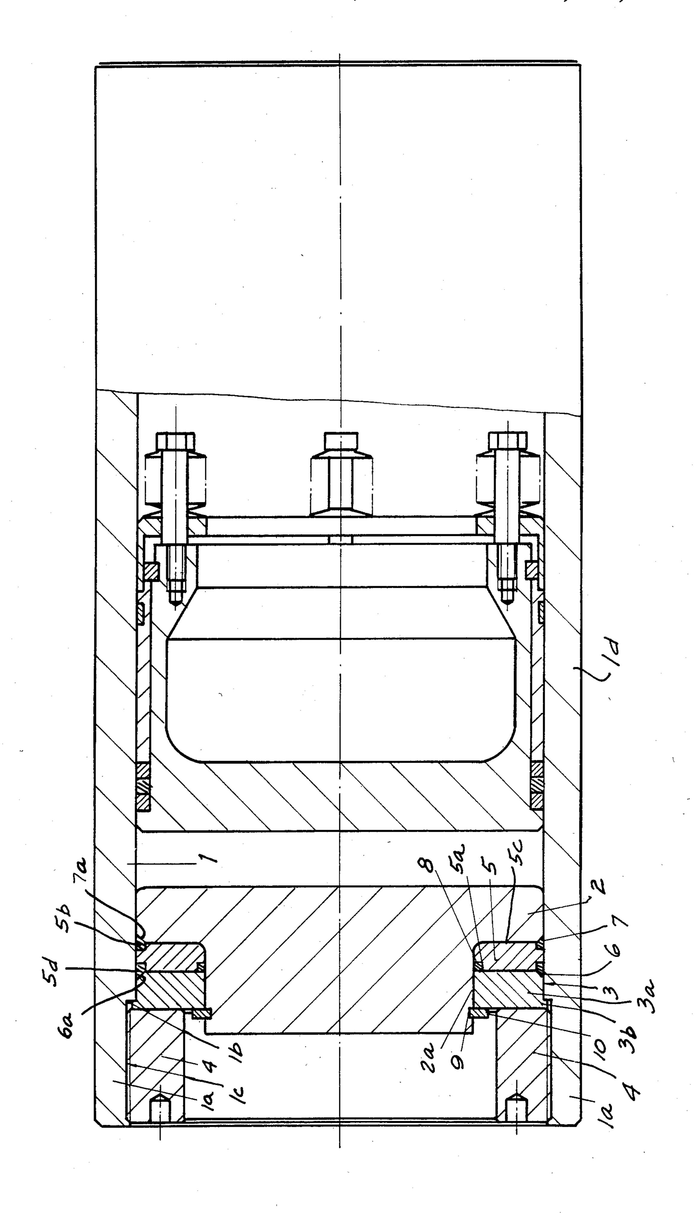
and this causes some diffuculties. Thus, the sealing ring will considerably be deformed thereby exposing the cylinder walls to a considerable radial pressure which could lead to a bulging out of the cylinder.
