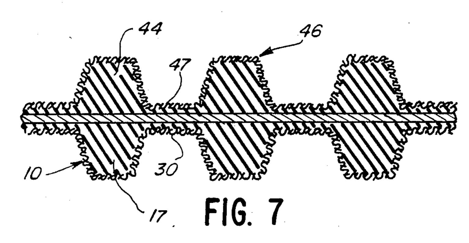
The preform, in the illustrated embodiment, is formed about a peripherally grooved cylindrical mold.
