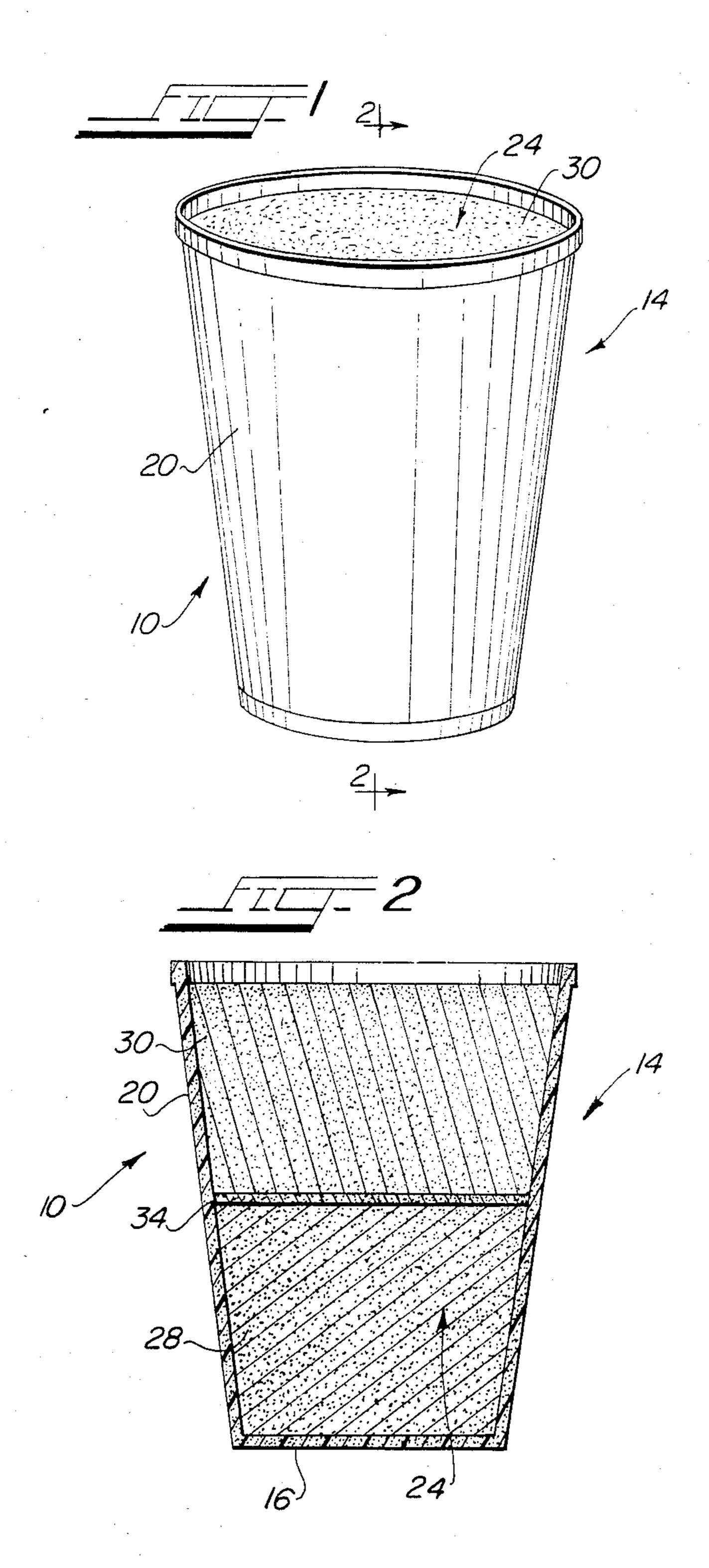
STAGED DETERGENT/FABRIC TREATING PREPARATION FOR USE IN WASHING MACHINES
