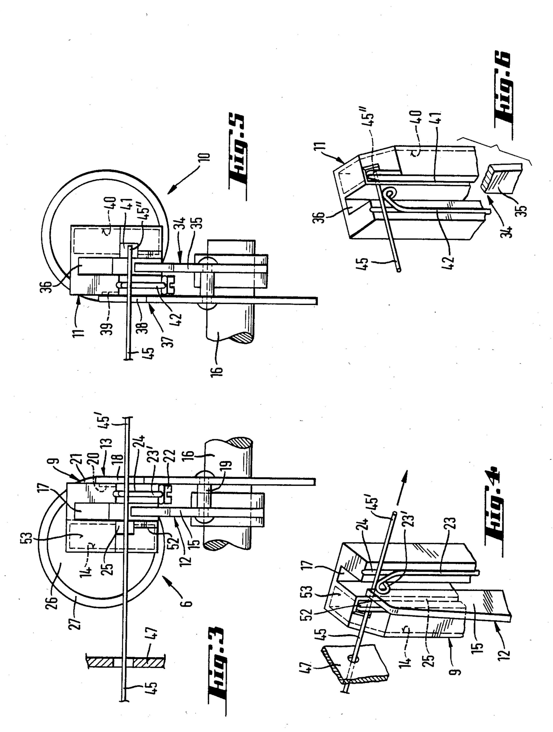
WEFT YARN CONTROL FOR A WEAVING MACHINE ROTOR
