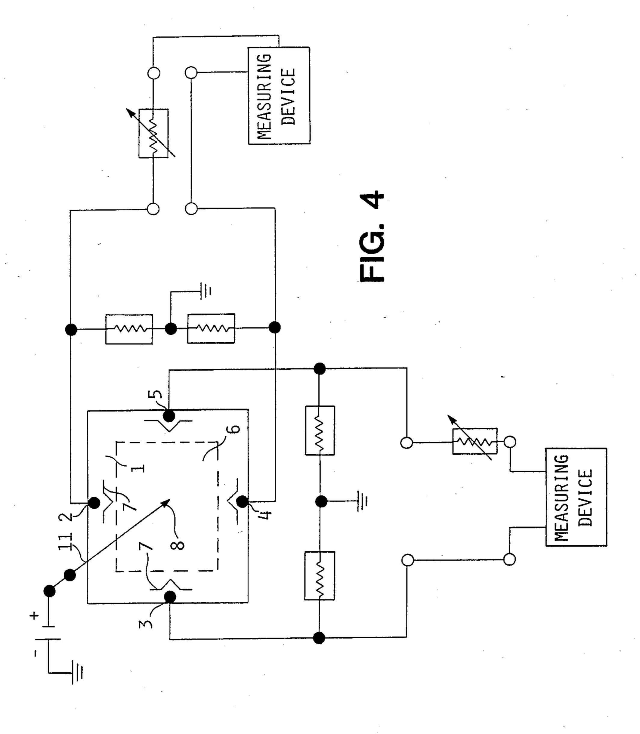
MEASURING DEVICE FOR DETERMINING THE LOCATION OF A STYLUS
