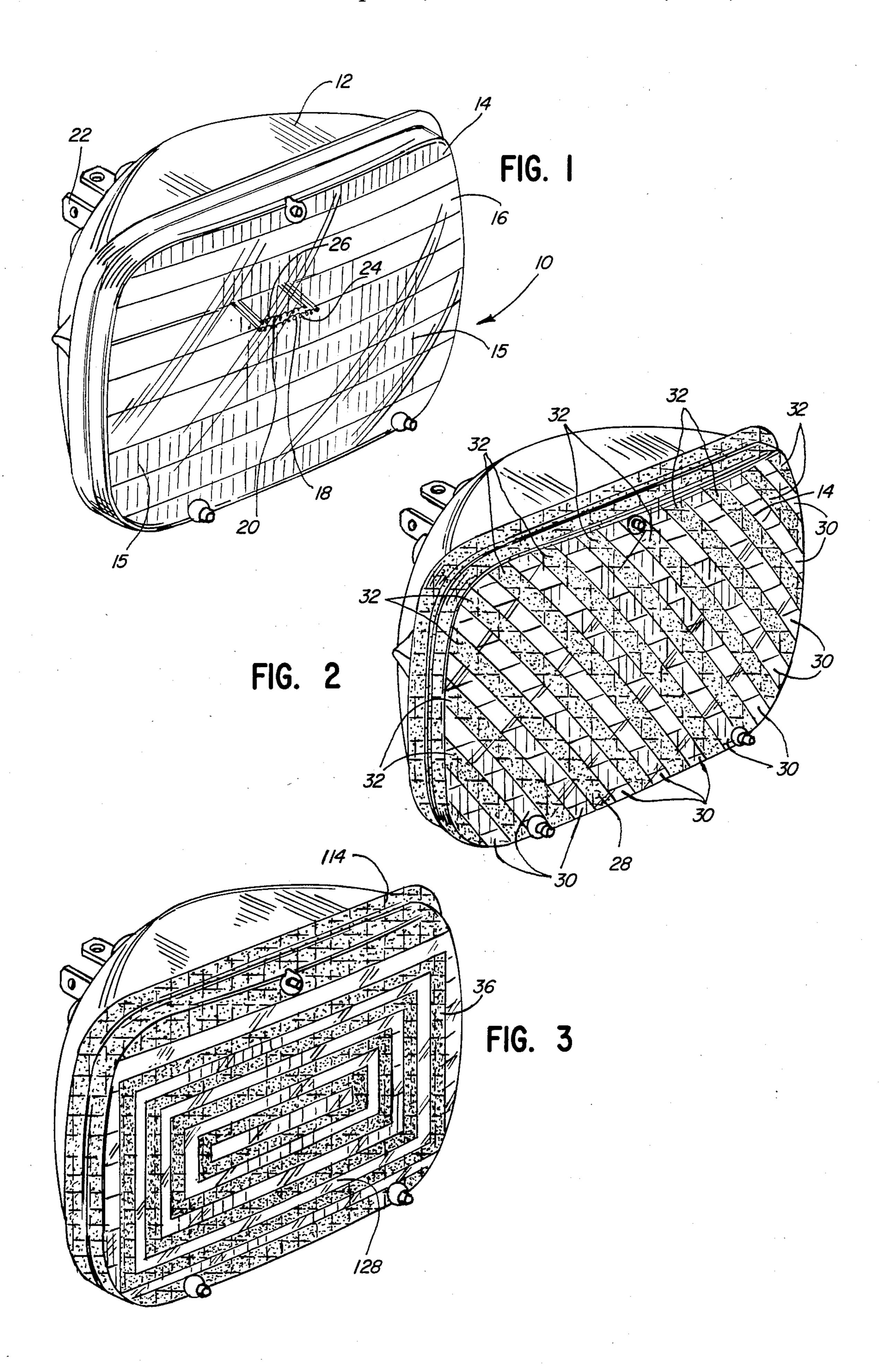
FIG. 2 is a perspective view of the lamp of FIG. 1 improved according to the present invention; and
