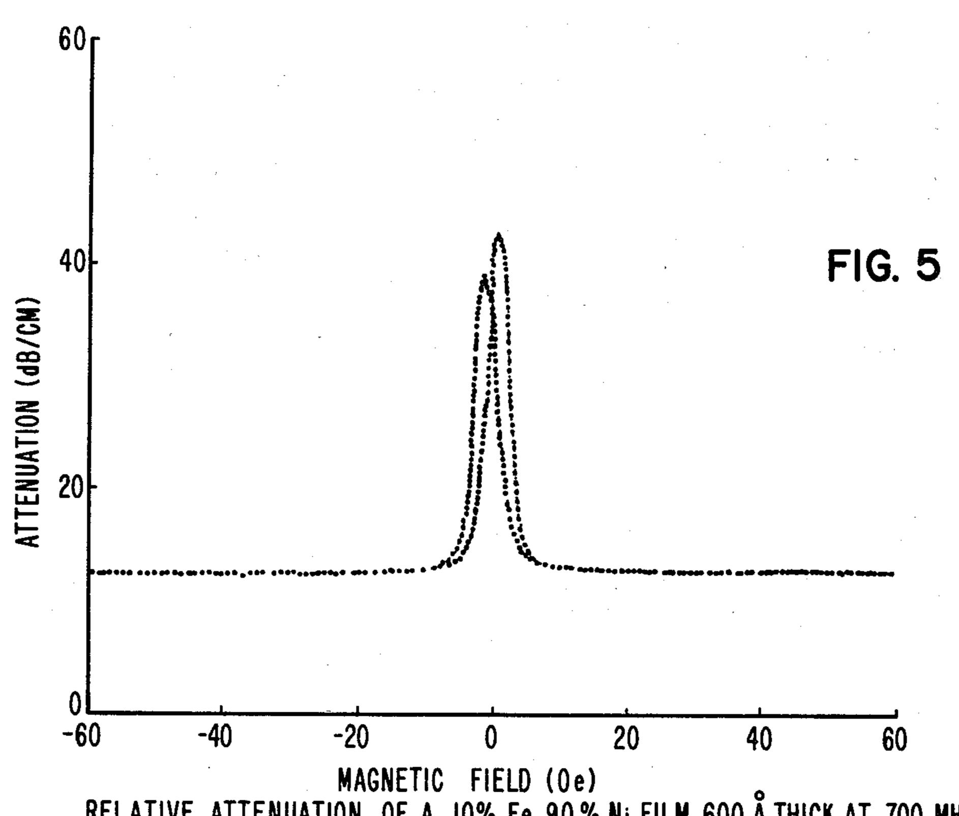
RELATIVE ATTENUATION OF A 10% Fe, 90% Ni FILM, 600 Å THICK AT 700 MHz
