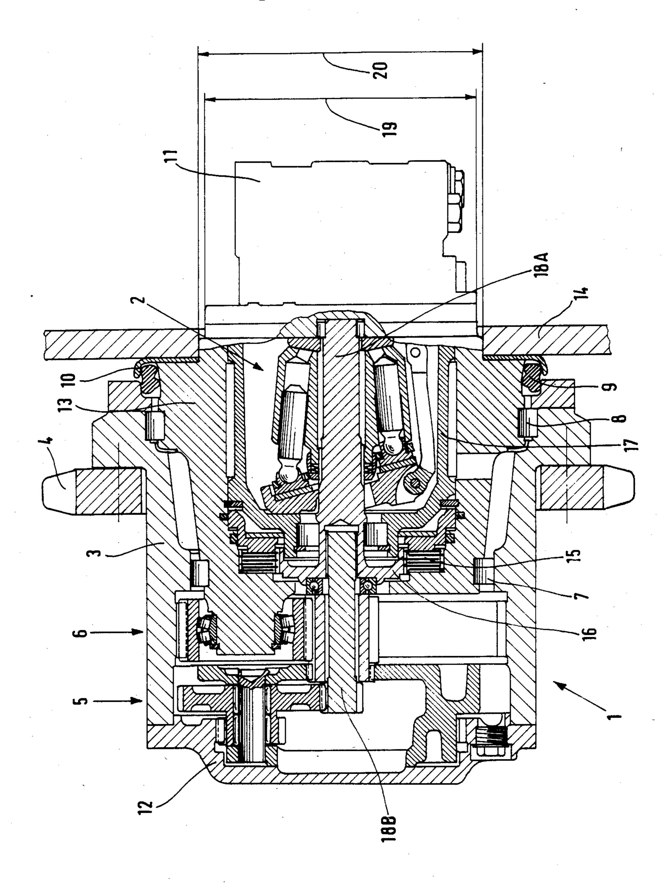
COMPACT HYDRAULIC DRIVE MECHANISM FOR WHEEL ASSEMBLIES
