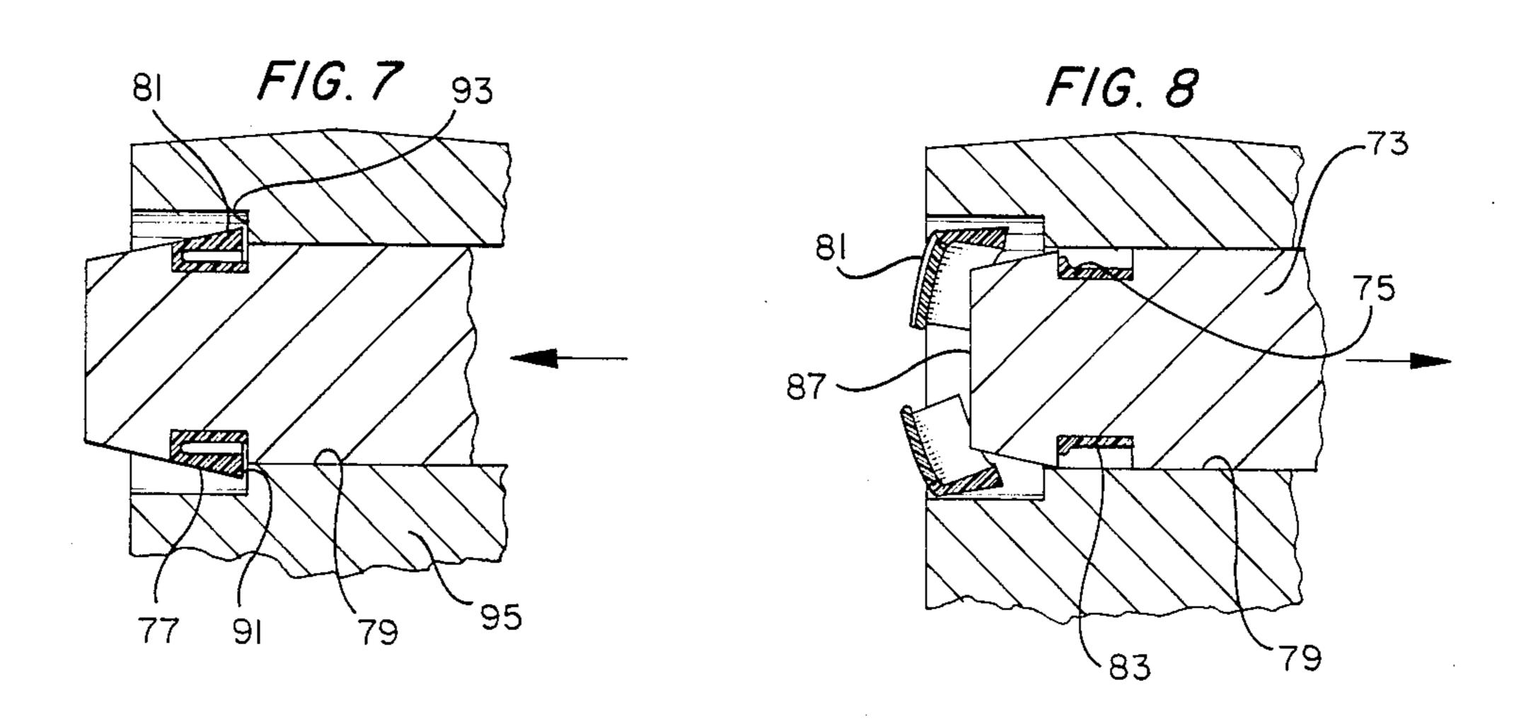
SHEAR LOCK KEEPER RING erv.
