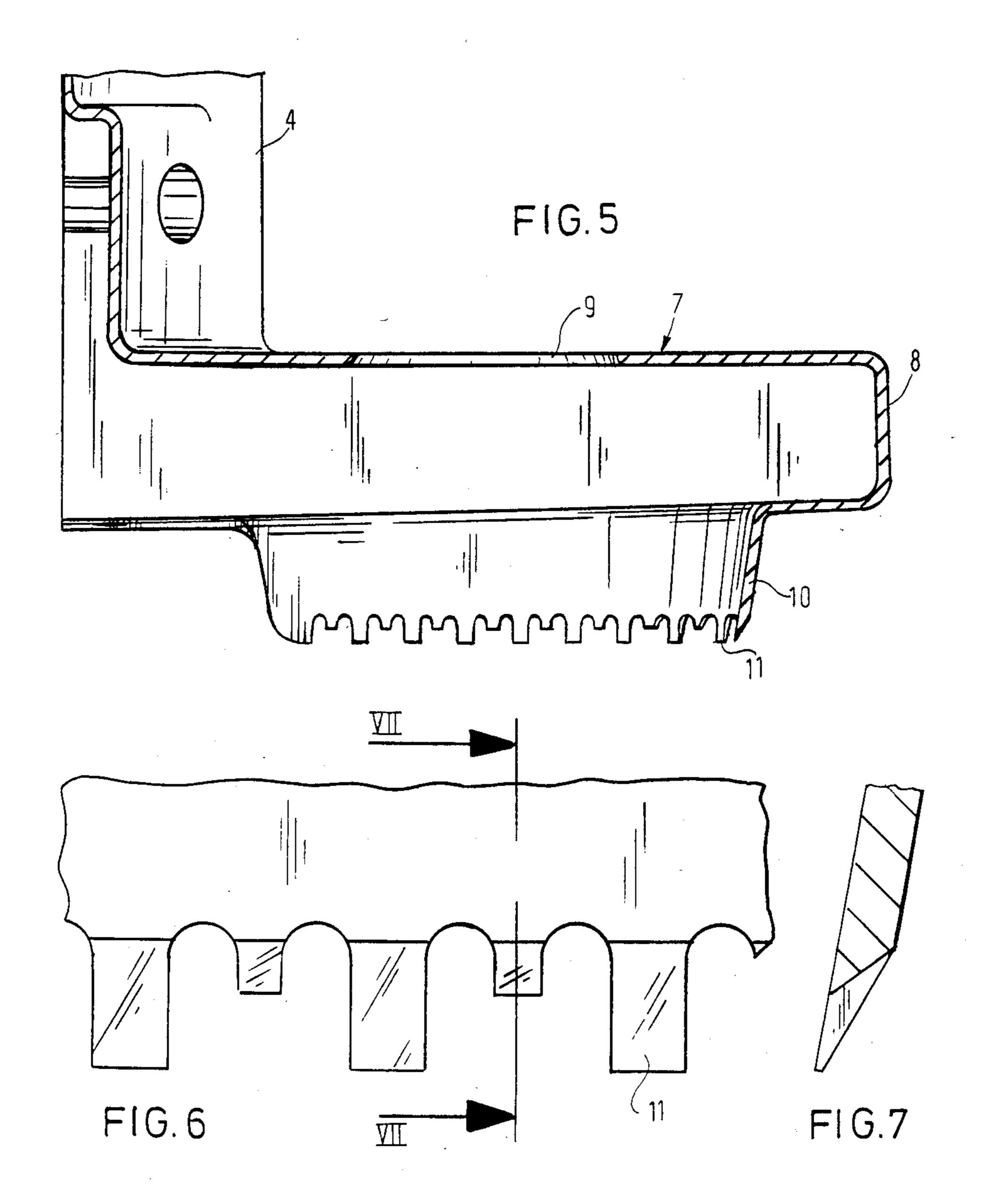
FIG. 6 shows a detail view of the ripping edge in FIG. 5,
