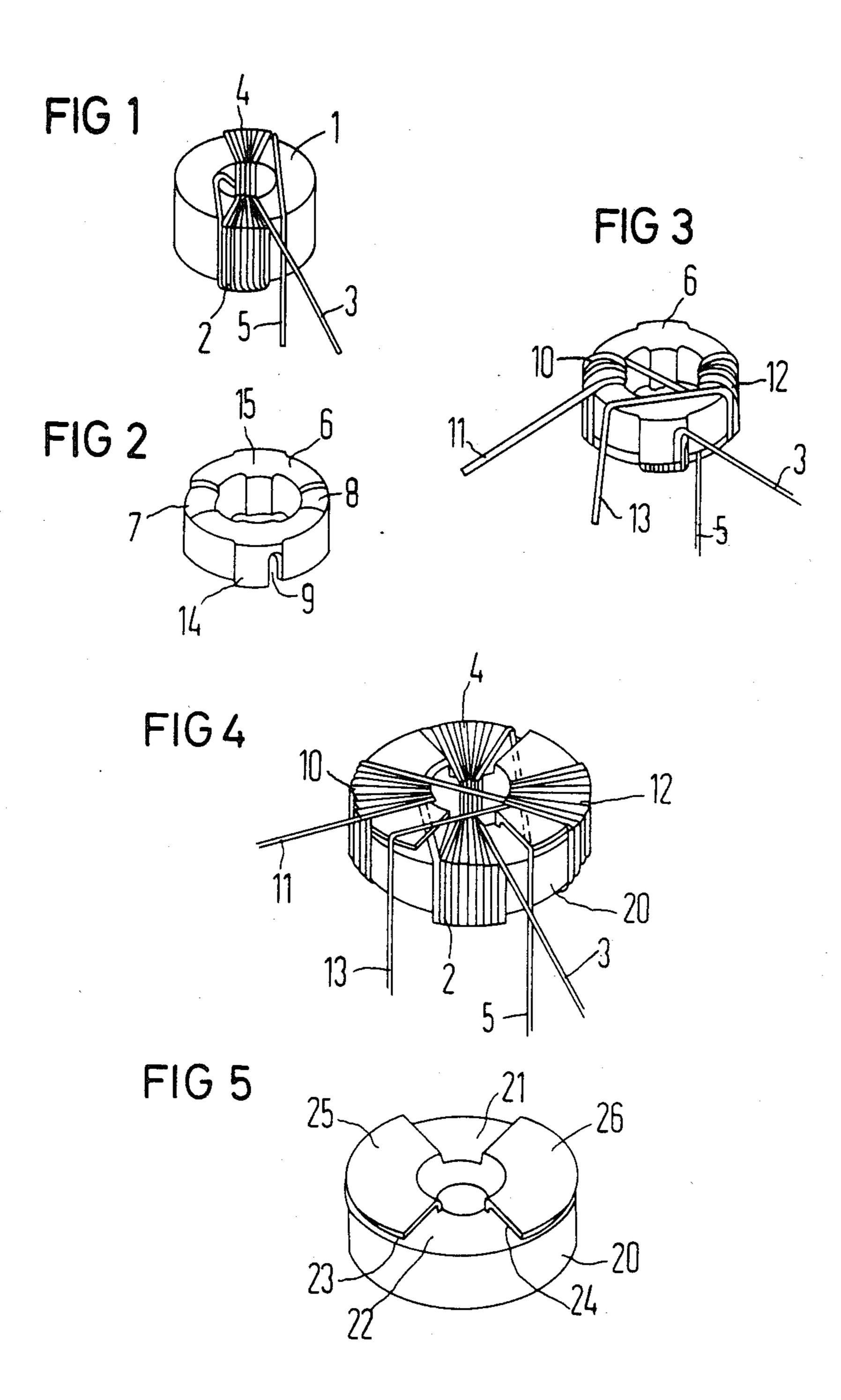
RADIO INTERFERENCE SUPPRESSION CHOKE WITH A LOW LEAKAGE FIELD
