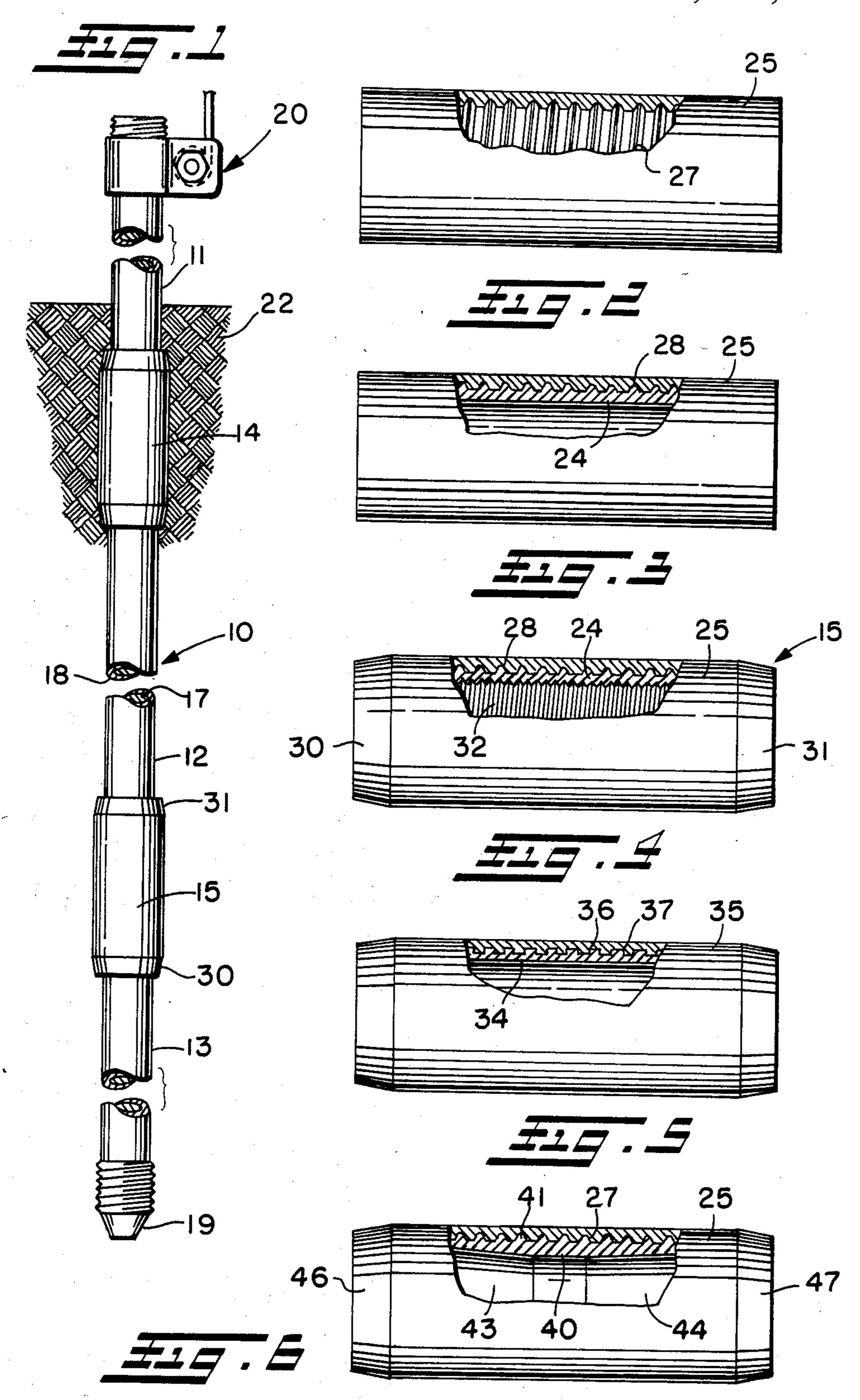
GROUND RODThis invention relates generally as indicated to a ground rod, coupling therefor, and method of making such coupling.
