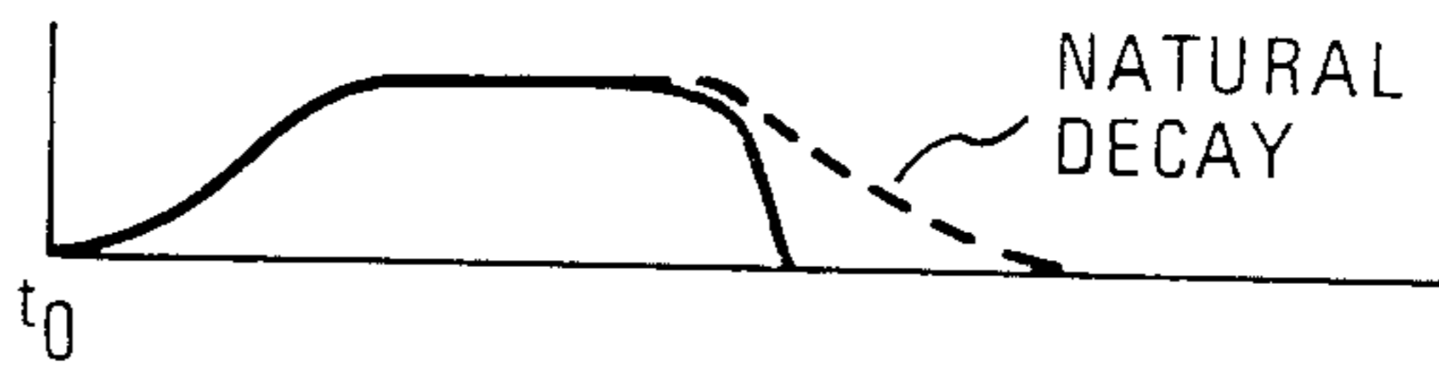
FIG. 4B OPTICAL GAIN IN LASER GAIN MEDIUM
