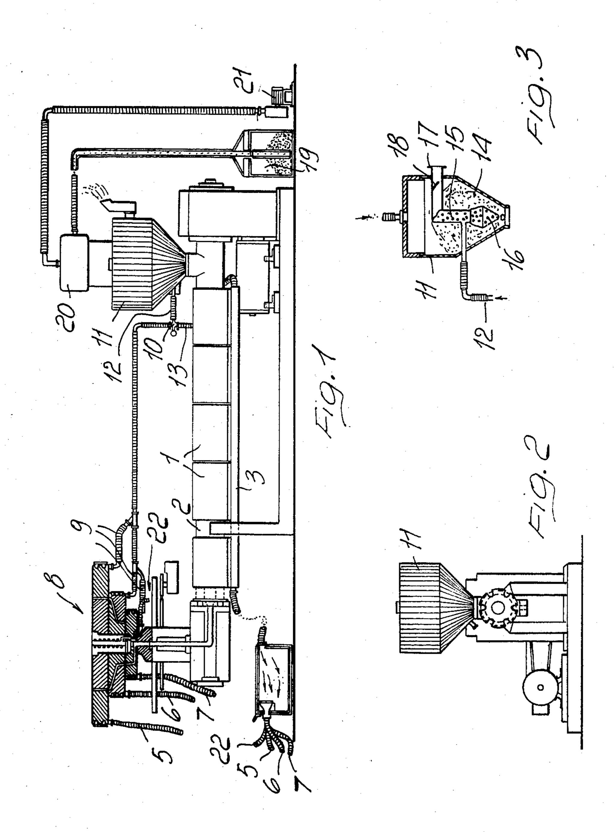
SYSTEM FOR HOT EXTRUDING, DRAWING, AND SIMILARLY PROCESSING PLASTOMERS OR ELASTOMERS, INCORPORATING A MEANS OF RECOVERING AND UTILIZING HEATED AIR FROM THE COOLING OF HEATED PARTS
