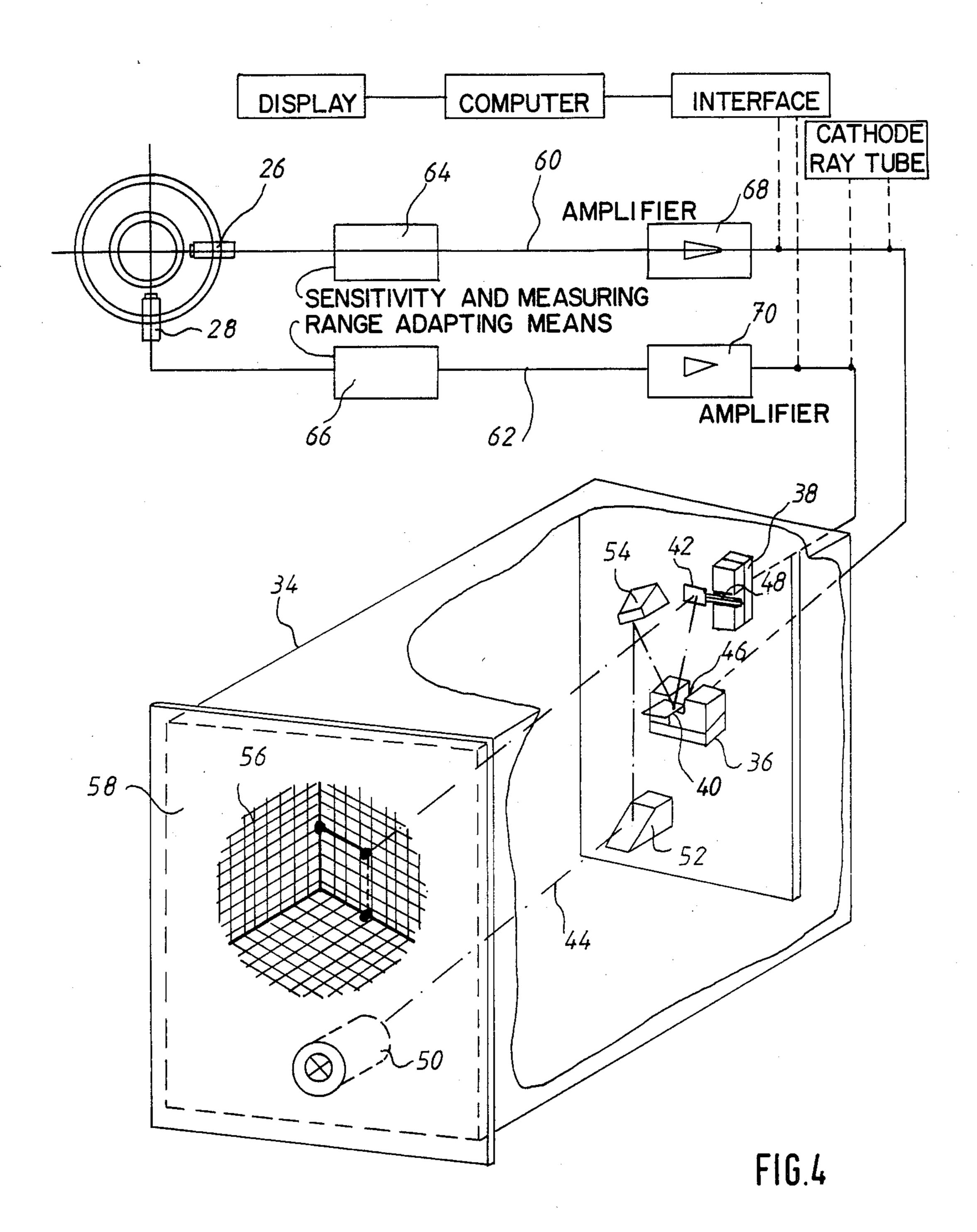
DEVICE FOR THE DETERMINATION OF THE UNBALANCE OF PROPELLERS
