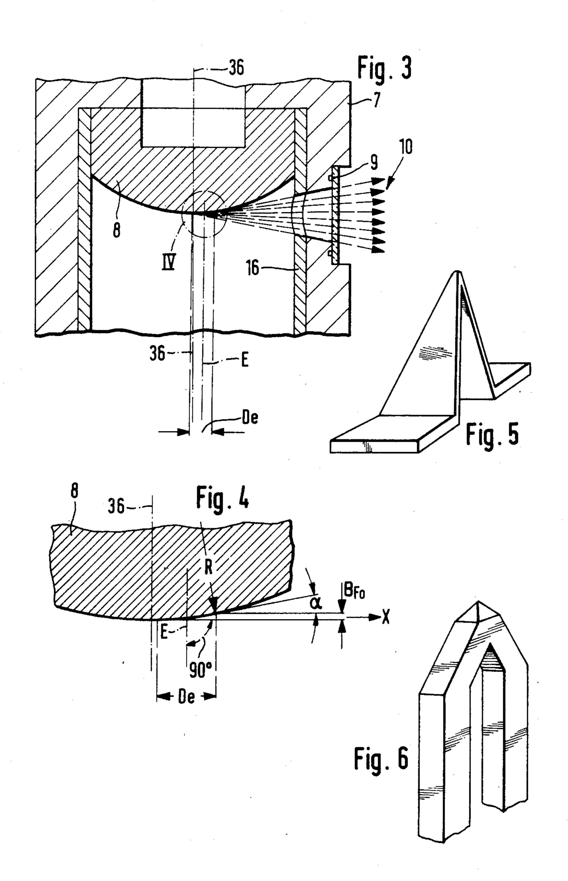
FINE FOCUS X-RAY TUBE AND METHOD OF FORMING A MICROFOCUS OF THE ELECTRON EMISSION OF AN X-RAY TUBE HOT CATHODE
