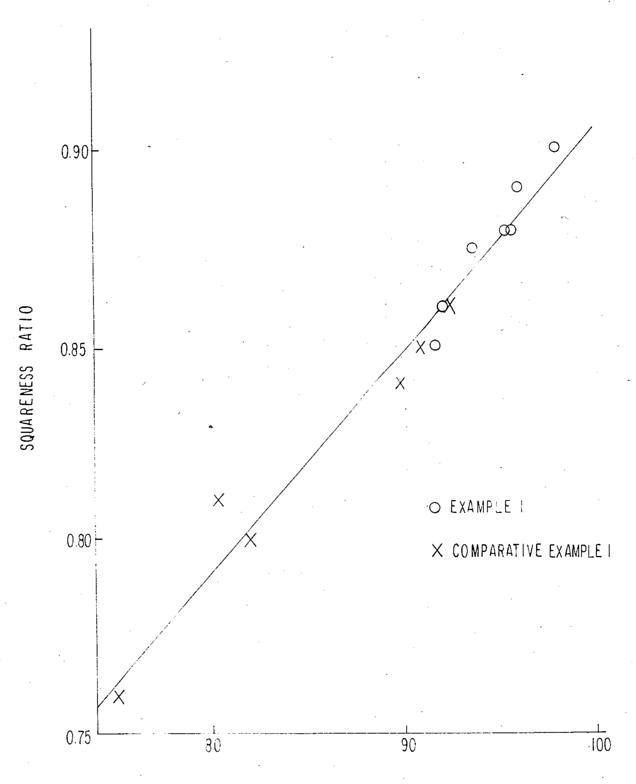
AMOUNT OF VINYL CHLORIDE COMPONENT IN COPOLYMER (wt%)
