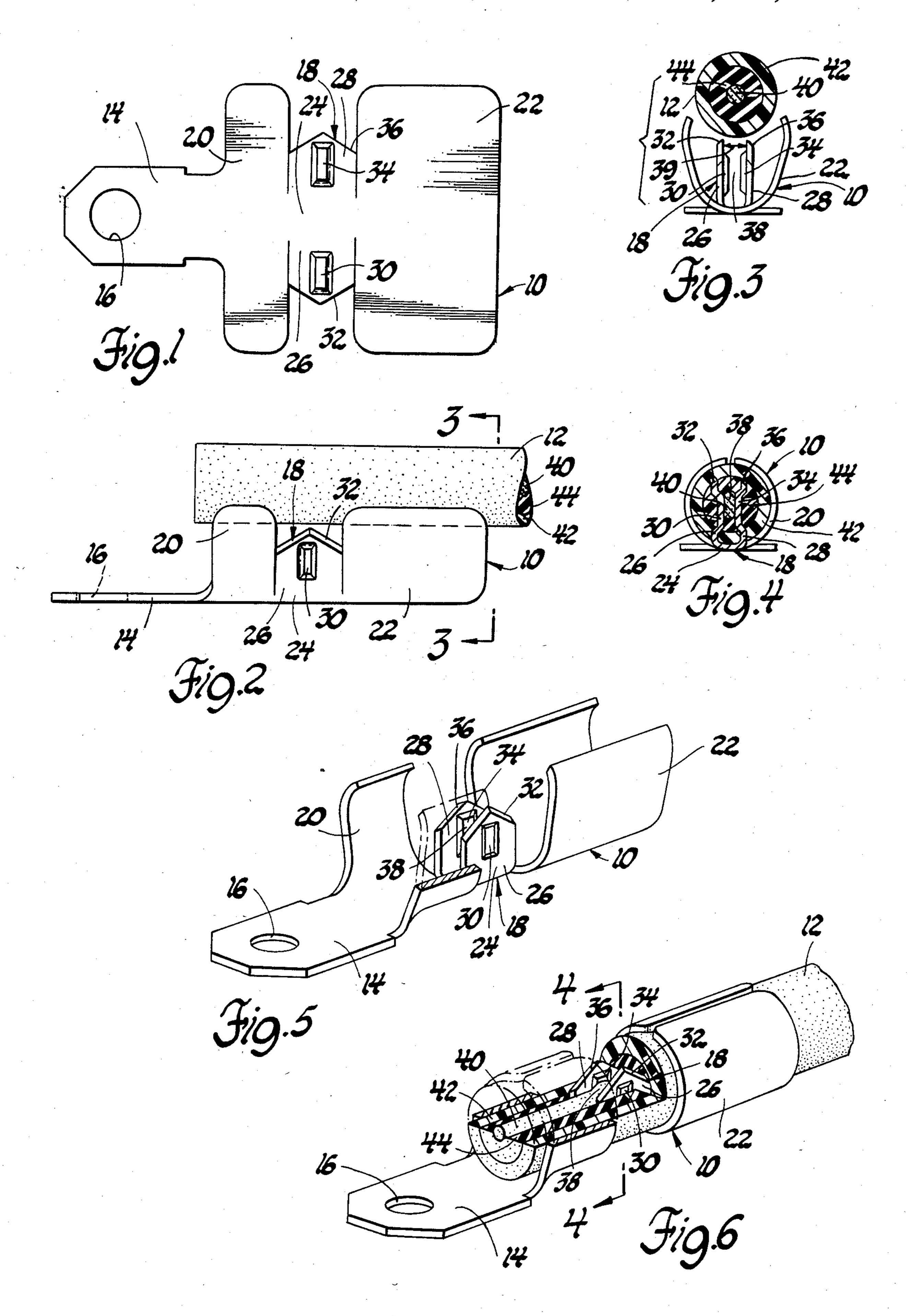
FIG. 3 is an end view of the insulation displacement terminal taken substantially along the line 3—3 of FIG.
