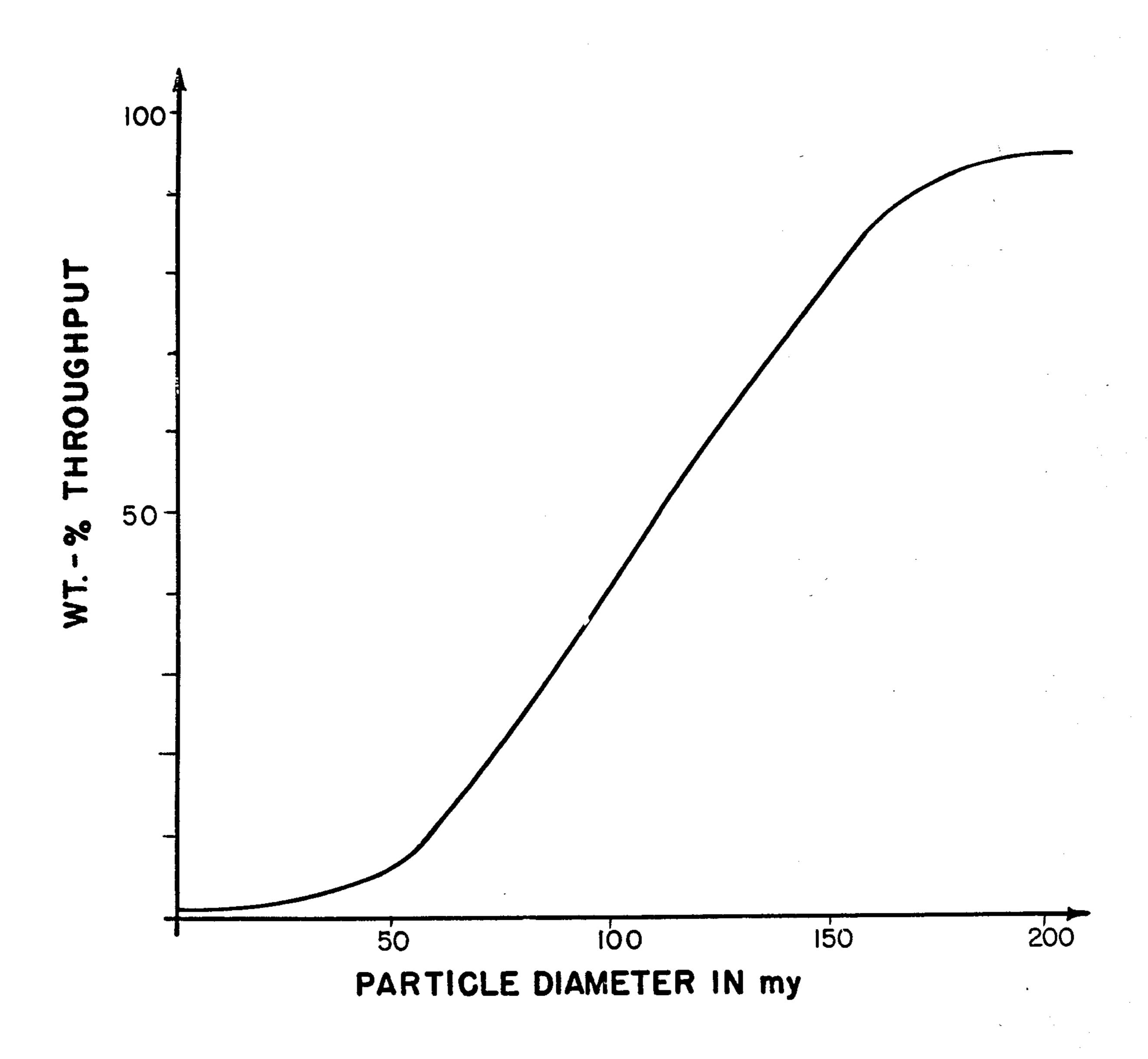
Fig.1 PARTICLE ANALYSIS COULTER COUNTER
