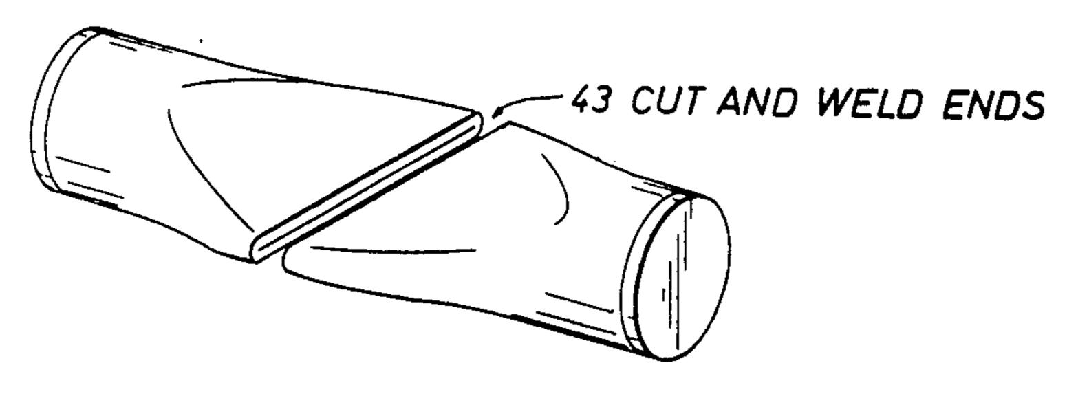
C. CUT PIPE IN HALF AND WELD SHUT THE ENDS.
