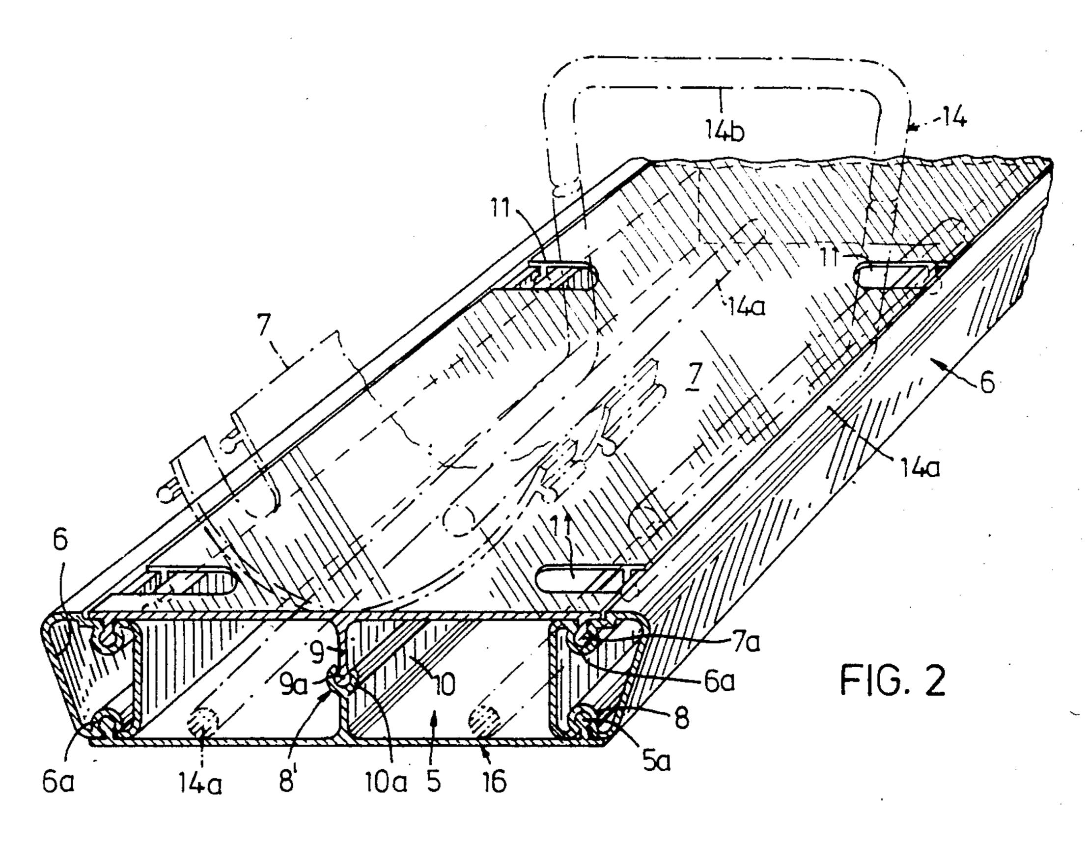
The invention starts from a holder of connecting bars for providing a positive connection of one structural member to another structural member to be concreted previously, with a basic part in which first sections of the connecting bars, to be connected to the one structural member, are accommodated, and a part covering these first sections and detachably connected to the basic part.
