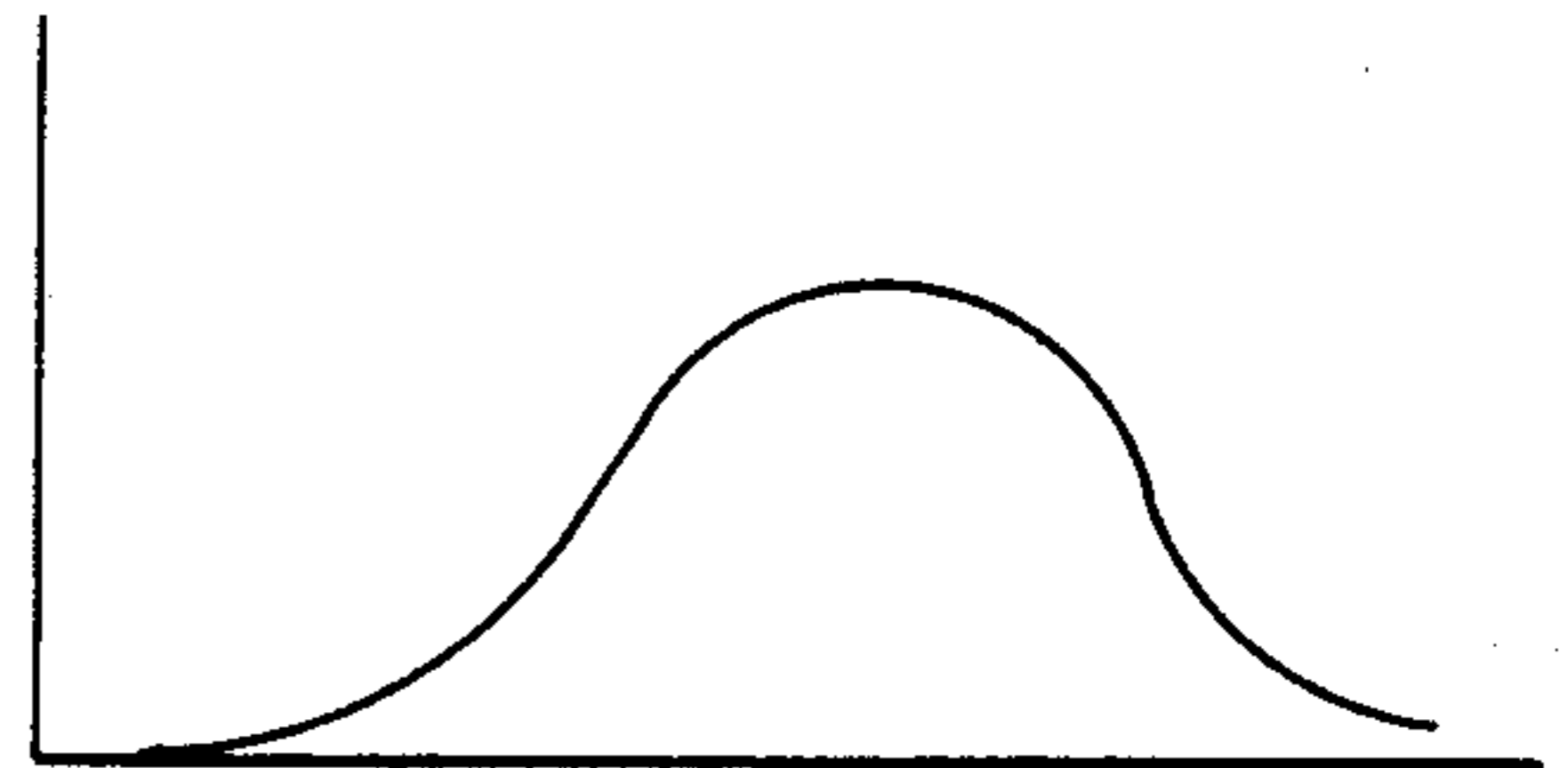
EDGE IMAGE ON ARRAY 360 DEFOCUSSED CONDITION, CONTACT 301 FULLY COMPRESSED IN Z AXIS DUE TO PART CONTACT
