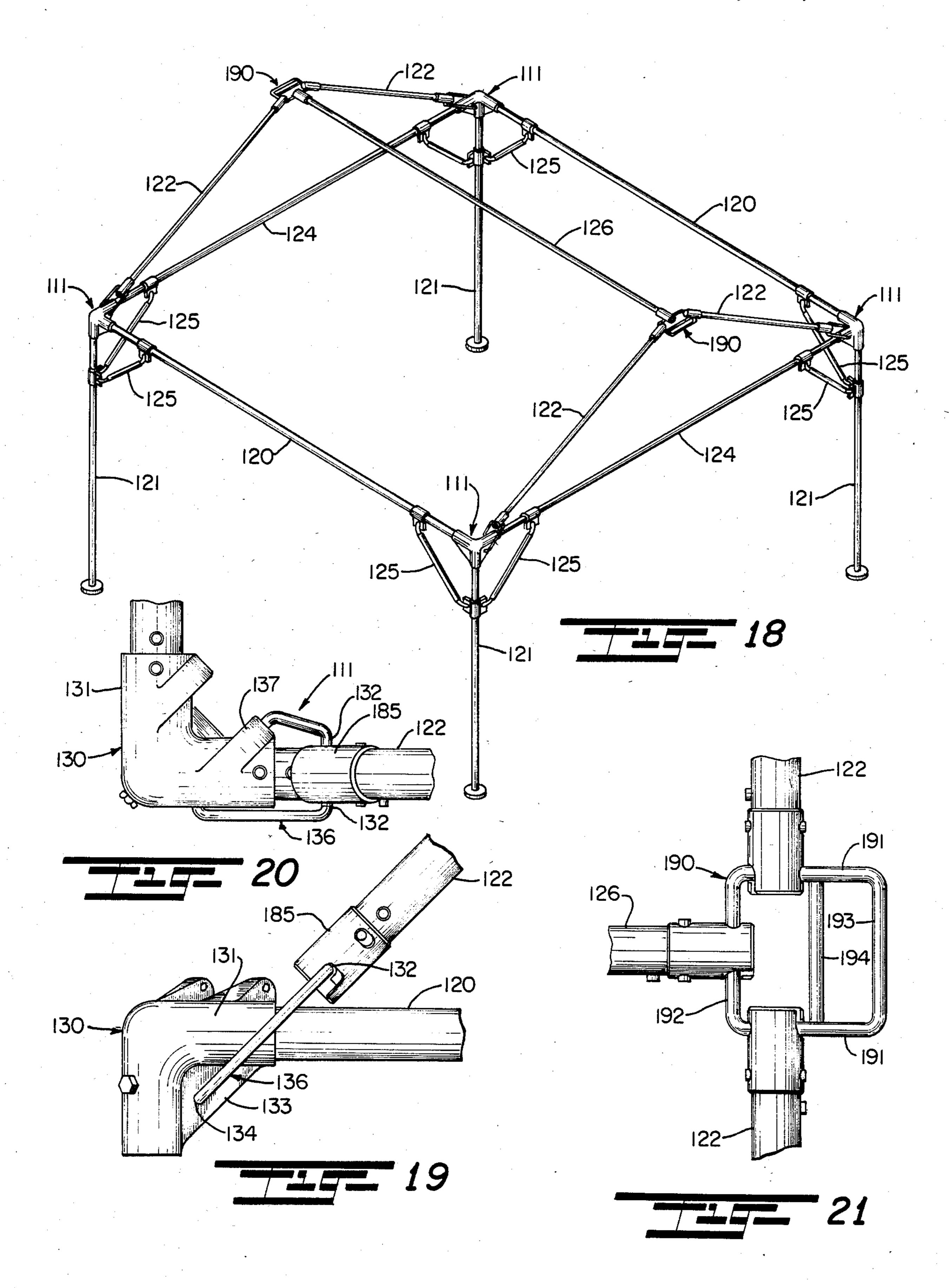
FRAME SYSTEM AND CONNECTORS FOR PORTABLE SHELTERS
