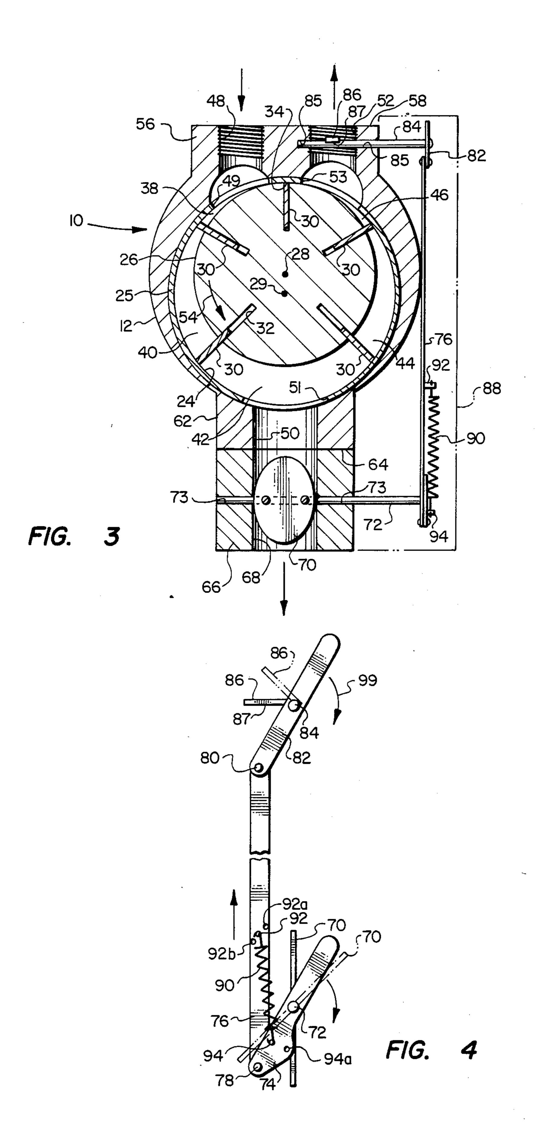
FLOW SENSING SPEED CONTROL FOR PRESSURE FLUID MOTOR
